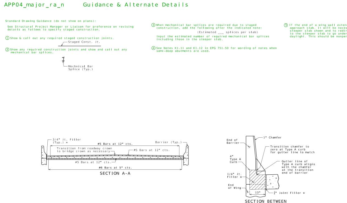
ALTERNATE DETAILS FOR TYPE B BARRIER (SBC)
