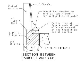
ALTERNATE DETAILS FOR TYPE B BARRIER (SBC)
