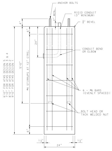
(4) AT THE OPTION OF THE CONTRACTOR THE CONCRETE FOUNDATIONS MAY BE PRECAST. IF PRECAST, THEY SHALL BE SET IN DRILLED HOLES 3 FEET IN DIAMETER AND 6 INCHES DEEPER THAN THE BOTTOM OF THE CONCRETE FOUNDATION. THE BOTTOM 6 INCHES OF THE HOLE AND THE REMAINING SPACE AROUND THE FOUNDATION SHALL BE BACKFILLED WITH WET TAMPED LIMESTONE SCREENINGS IN LAYERS NOT EXCEEDING 12 INCHES.
