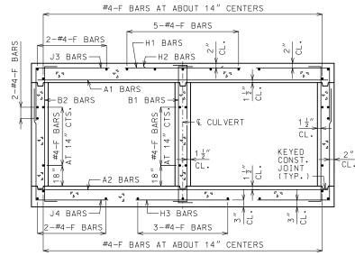
BARREL REINFORCEMENT FOR DESIGN FILLS OVER 2'-0"
