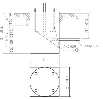
\* SURFACE OF BASE TO BE CONSTRUCTED SQUARE FOR A DEPTH OF 12".
