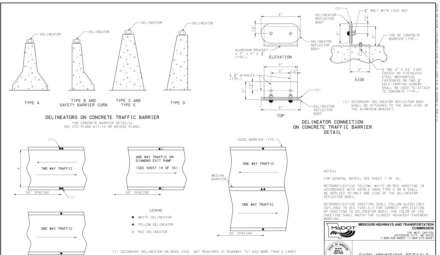
ROADWAY OR BRIDGE CONCRETE TRAFFIC BARRIER DELINEATION
