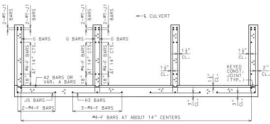
UPSTREAM AND DOWNSTREAM WINGS REINFORCEMENT
