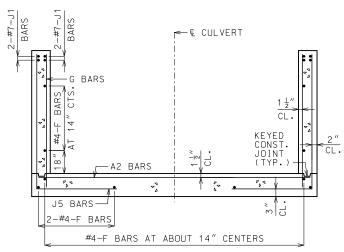
UPSTREAM AND DOWNSTREAM WINGS REINFORCEMENT
