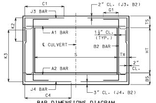
BAR DIMENSIONS DIAGRAM SYMMETRICAL ABOUT & CULVERT.
