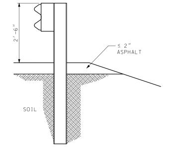
SETTING POST THROUGH ASPHALT ≤ 2" THICK
