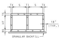
GRANULAR BACKFILL LIMITS AND MEMBER DIMENSIONS
