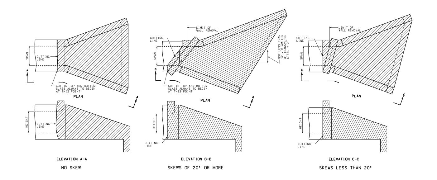
THE HATCHED PARTS OF THESE DRAWINGS INDICATE THOSE PORTIONS OF THE EXISTING CULVERT WHICH ARE TO BE REMOVED.
