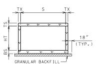
GRANULAR BACKFILL LIMITS AND MEMBER DIMENSIONS
