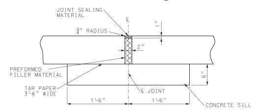
SILL SHALL EXTEND 18" BEYOND EACH EDGE OF THE PAVEMENT AND SHALL BE CONSTRUCTED OF CONCRETE REGARDLESS OF ADJACENT BASE MATERIAL.
