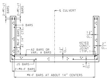
UPSTREAM AND DOWNSTREAM WINGS REINFORCEMENT
