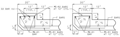
UPSTREAM HEADWALL REINFORCEMENT NEAR INTERIOR WALL
