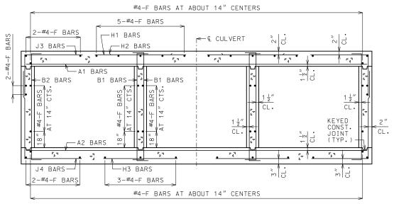
BARREL REINFORCEMENT FOR DESIGN FILLS OVER 2'-0"
