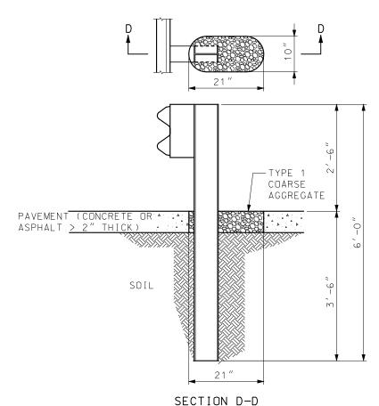
SETTING POST THROUGH PAVEMENT (CONCRETE OR ASPHALT > 2" THICK)
