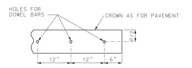
PART ELEVATION OF HEADER PLANK
