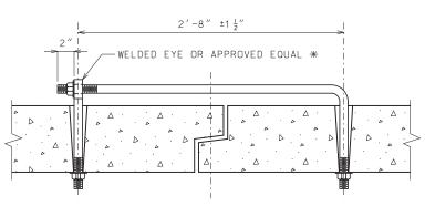
\* THE CONNECTIONS SHALL BE PLACED AT DOWNSTREAM END WHEN PLACED INSIDE OF STRUCTURE. EYE BOLT TIE OPTION
