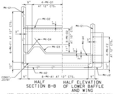
NOTE: BEND OR CUT D1 BARS IN FIELD TO CLEAR NOTCH IN BAFFLE WALL.
