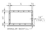
GRANULAR BACKFILL LIMITS AND MEMBER DIMENSIONS
