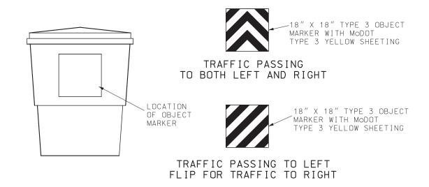
TYPE 3 OBJECT MARKER PLACEMENT FOR PERMANENT INSTALLATIONS
