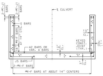
UPSTREAM AND DOWNSTREAM WINGS REINFORCEMENT
