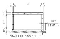
GRANULAR BACKFILL LIMITS AND MEMBER DIMENSIONS
