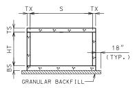
GRANULAR BACKFILL LIMITS AND MEMBER DIMENSIONS
