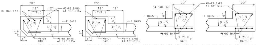
UPSTREAM HEADWALL REINFORCEMENT
