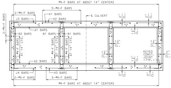
BARREL REINFORCEMENT FOR DESIGN FILLS OVER 2'-0"
