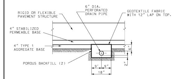
SECTION D-D WITH PERMEABLE BASE
