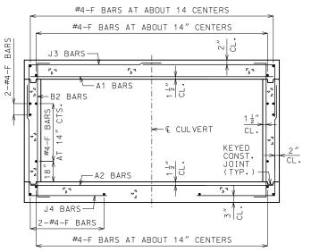
BARREL REINFORCEMENT FOR DESIGN FILLS 2'-0" OR LESS
