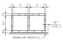
GRANULAR BACKFILL LIMITS AND MEMBER DIMENSIONS
