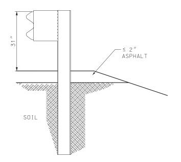
SETTING POST THROUGH ASPHALT ≤ 2" THICK
