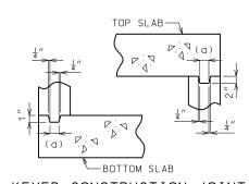
KEYED CONSTRUCTION JOINT (a) APPROXIMATELY ONE-THIRD OF WALL THICKNESS
