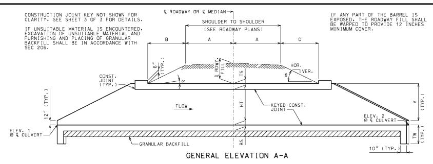
CHANNEL BOTTOM SHALL BE GRADED WITHIN RIGHT OF WAY FOR TRANSITION OF CHANNEL BED TO CULVERT OPENINGS. CHANNEL BANKS SHALL BE TAPERED TO MATCH CULVERT OPENINGS.
