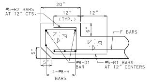
UPSTREAM HEADWALL REINFORCEMENT
