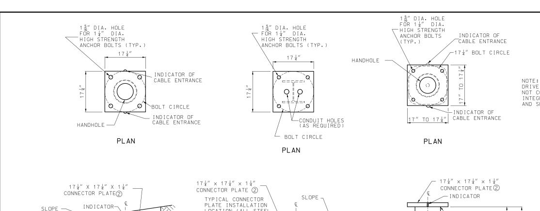
DRIVE HOLES WILL BE PERMITTED PROVIDED THEY DO NOT CONFLICT WITH OR COMPROMISE THE STRUCTURAL INTEGRITY OF THE PLATE, THE WELD BETWEEN THE PLATE AND SHAFT, OR THE BOLT HOLES.
