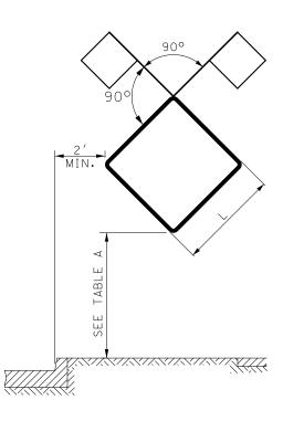
HEIGHT AND LATERAL LOCATIONS FOR POST AND PORTABLE SIGN MOUNTING
