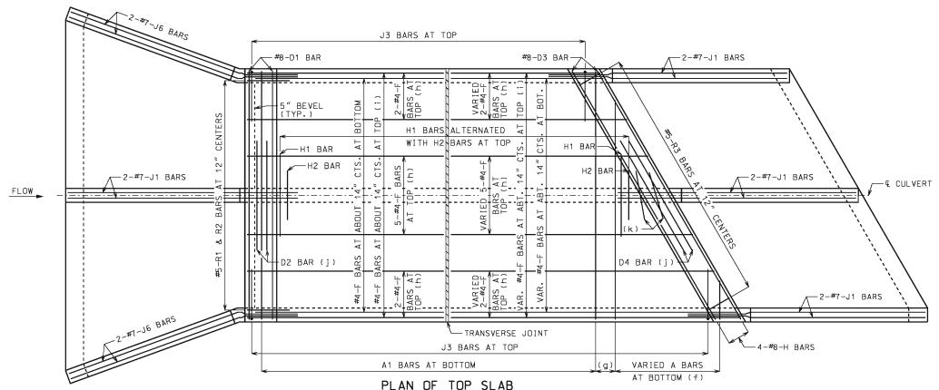
B BARS IN WALLS ARE NOT SHOWN FOR CLARITY, FOR PLACEMENT, SEE SHEET 1 OF 3.
