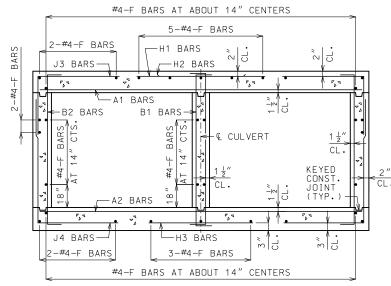
BARREL REINFORCEMENT FOR DESIGN FILLS OVER 2'-0"
