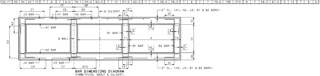
IF DESIGN FILL IS BETWEEN TABULATED DESIGN FILLS, USE THE NEXT GREATER TABULATED DESIGN FILL, EXCEPT FOR DESIGN FILLS BETWEEN 2 FEET AND 4 FEET. FOR DESIGN FILLS BETWEEN 2 FEET AND 4 FEET USE THE GREATER MEMBER THICKNESS, AREA OF REINFORCEMENT AND BAR DIMENSIONS FROM THE 2 FEET AND 4 FEET TABULATED DESIGN FILLS. AREA OF REINFORCEMENT EQUALS BAR AREA PER FOOT SPACING.
