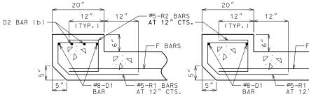
UPSTREAM HEADWALL REINFORCEMENT NEAR INTERIOR WALL
