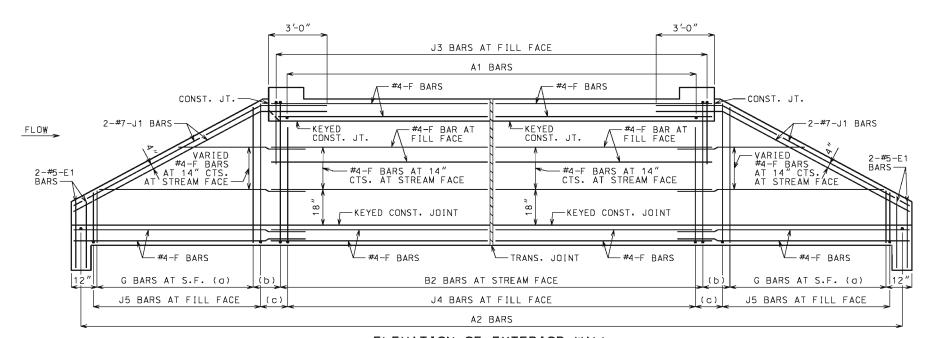
ELEVATION OF EXTERIOR WALL J1 BARS MAY BE BENT IN FIELD OR SHOP.
