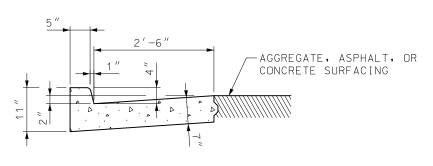
SECTION THRU CONCRETE CURB AND GUTTER
