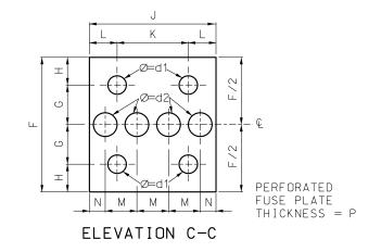
ALL HOLES SHALL BE DRILLED. ALL PLATE CUTS SHALL PREFERABLY BE SAW CUTS. HOWEVER: FLAME CUTTING WILL BE PERMITTED PROVIDED ALL EDGES ARE GROUND.
