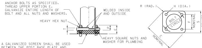
BETWEEN THE POST BASE PLATE AND CONCRETE BASE, SCREENS SHALL BE PRESS-FORMED OF 3 OR 4 MESH. 21 GAGE OR HEAVIER. STAINLESS STEEL OR HOT-DIPPED GALVANIZED WIRE SCREEN OR APPROVED EQUIVALENT. THAT WILL PROVIDE A FRICTION-TIGHT FIT WHEN INSTALLED.
