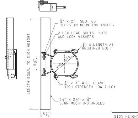
NOTE: MINIMUM OF TWO BRACKETS ARE REQUIRED FOR SIGNS OVER 42" IN LENGTH.
