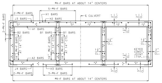
BARREL REINFORCEMENT FOR DESIGN FILLS OVER 2'-0"
