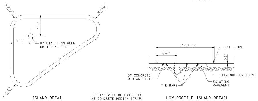
GENERAL NOTES: FOR DETAILS ON CONCRETE MEDIAN STRIP CONSTRUCTION, SEE STANDARD PLAN 608.30.
