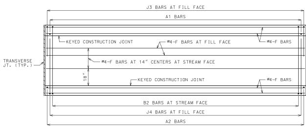
ELEVATION OF WALL REINFORCEMENT
