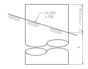
TYPE A (FILL) (FOR ADDITIONAL DETAILS SEE TYPE A FLAT GROUND)
