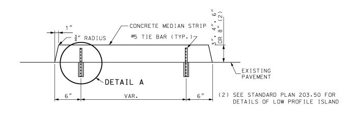
SECTION A-A CONCRETE MEDIAN STRIP
