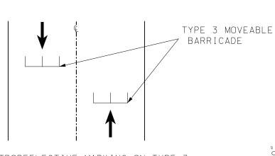
RETROREFLECTIVE MARKING ON TYPE 3 BARRICADES SHALL BE ON BOTH SIDES OF EACH RAIL AND DIRECT TRAFFIC MOVEMENT APPROPRIATELY TO ALLOW VEHICLES TO PASS THROUGH
