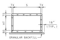
GRANULAR BACKFILL LIMITS AND MEMBER DIMENSIONS
