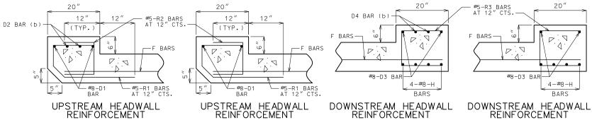
(b) #8 FOR CLEAR SPAN > 10'-0" #9 FOR CLEAR SPAN > 13'-0'
