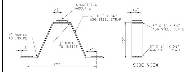
DETAILS OF TYPE F TEMPORARY BARRIER TIE-DOWN STRAP
