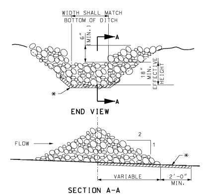
\* GEOTEXTILE LINING MAY BE INSTALLED AS REQUIRED BY THE ENGINEER.
