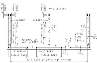
UPSTREAM AND DOWNSTREAM WINGS REINFORCEMENT
