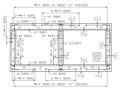
BARREL REINFORCEMENT FOR DESIGN FILLS OVER 2'-0"
