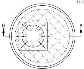
PLAN OF FLAT SLAB MANHOLE TOP
