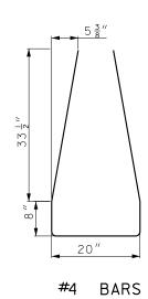
CONCRETE BARRIER END ANCHORAGE ON GRADE
