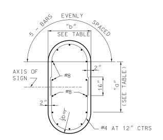
SECTION A-A (TYPICAL SECTION SHOWING REINFORCING STEEL)
