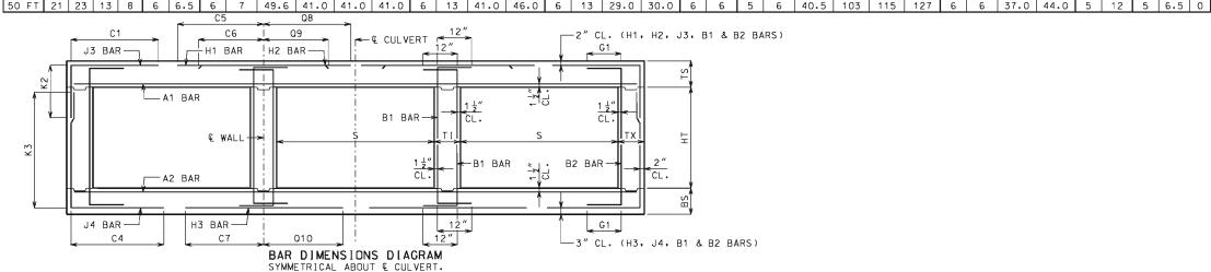
IF DESIGN FILL IS BETWEEN TABULATED DESIGN FILLS, USE THE NEXT GREATER TABULATED DESIGN FILL, EXCEPT FOR DESIGN FILLS BETWEEN 2 FEET AND 4 FEET. FOR DESIGN FILLS BETWEEN 2 FEET AND 4 FEET USE THE GREATER MEMBER THICKNESS, AREA OF REINFORCEMENT AND BAR DIMENSIONS FROM THE 2 FEET AND 4 FEET TABULATED DESIGN FILLS. AREA OF REINFORCEMENT EQUALS BAR AREA PER FOOT SPACING.
