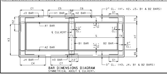
IF DESIGN FILL IS BETWEEN TABULATED DESIGN FILLS, USE THE NEXT GREATER TABULATED DESIGN FILL, EXCEPT FOR DESIGN FILLS BETWEEN 2 FEET AND 4 FEET. FOR DESIGN FILLS BETWEEN 2 FEET AND 4 FEET USE THE GREATER MEMBER THICKNESS, AREA OF REINFORCEMENT AND BAR DIMENSIONS FROM THE 2 FEET AND 4 FEET TABULATED DESIGN FILLS. AREA OF REINFORCEMENT EQUALS BAR AREA PER FOOT SPACING.
