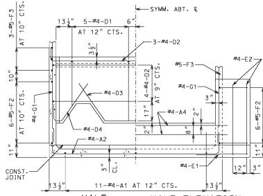
HALF HALF ELEVATION SECTION B-B OF LOWER BAFFLE AND WING
