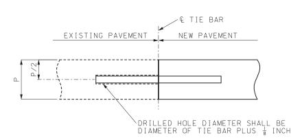
TIE BARS SHALL BE EPOXY COATED, DEFORMED REINFORCING BARS MEETING THE REQUIREMENTS OF SECTIONS 710 AND 1057.
