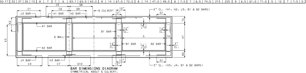
IF DESIGN FILL IS BETWEEN TABULATED DESIGN FILLS, USE THE NEXT GREATER TABULATED DESIGN FILL, EXCEPT FOR DESIGN FILLS BETWEEN 2 FEET AND 4 FEET. FOR DESIGN FILLS BETWEEN 2 FEET AND 4 FEET USE THE GREATER MEMBER THICKNESS, AREA OF REINFORCEMENT AND BAR DIMENSIONS FROM THE 2 FEET AND 4 FEET TABULATED DESIGN FILLS. AREA OF REINFORCEMENT EQUALS BAR AREA PER FOOT SPACING.
