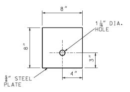
DETAIL OF STEEL BEARING PLATE
