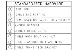
FOR ARRANGEMENT OF SPRING AND COMPENSATING CABLE END ASSEMBLIES AND TURNBUCKLE CABLE END ASSEMBLIES, THE FOLLOWING CRITERIA SHALL APPLY: LENGTH OF CABLE RUNS TO 1000' - USE COMPENSATING CABLE END ASSEMBLY ON ONE END AND THE TURNBUCKLE CABLE END ASSEMBLY ON THE OTHER END OF EACH INDIVIDUAL CABLE, FOR LENGTHS LONGER THAN 1000' AND UP TO AND INCLUDING 2000' - USE COMPENSATING CABLE END ASSEMBLY ON EACH END OF THE INDIVIDUAL CABLE.
