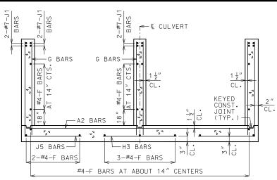
UPSTREAM AND DOWNSTREAM WINGS REINFORCEMENT
