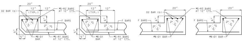
UPSTREAM HEADWALL REINFORCEMENT
