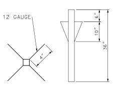
OMNI-DIRECTIONAL ANCHOR DETAIL FOR BOTH 12 AND 7 GAUGE
