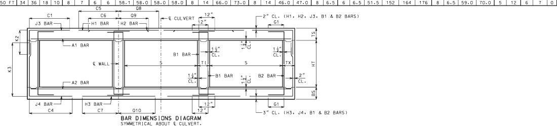
J IF DESIGN FILL IS BETWEEN TABULATED DESIGN FILLS, USE THE NEXT GREATER TABULATED DESIGN FILL, EXCEPT FOR DESIGN FILLS BETWEEN 2 FEET AND 4 FEET. FOR DESIGN FILLS BETWEEN 2 FEET AND 4 FEET USE THE GREATER MEMBER THICKNESS, AREA OF REINFORCEMENT AND BAR DIMENSIONS FROM THE 2 FEET AND 4 FEET TABULATED DESIGN FILLS.
