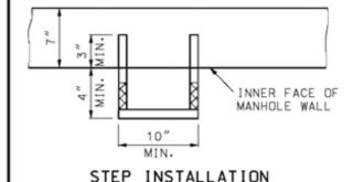
STEPS SHALL BE PLACED AT VERTICAL INTERVALS OF 16" MAXIMUM IN ALL MANHOLES HAVING A DEPTH OF MORE THAN 4'-0". STEPS SHALL BEGIN AT AN ELEVATION 6" ABOVE THE TOP OF THE OUTLET PIPE.
