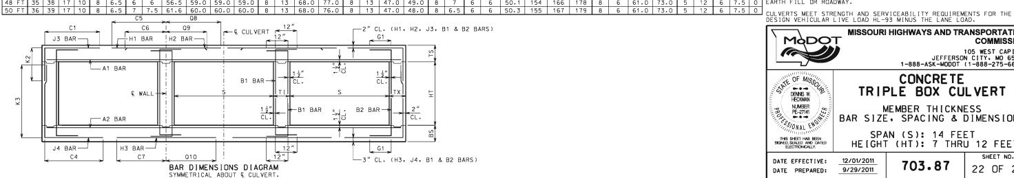
IF DESIGN FILL IS BETWEEN TABULATED DESIGN FILLS, USE THE NEXT GREATER TABULATED DESIGN FILL, EXCEPT FOR DESIGN FILLS BETWEEN 2 FEET AND 4 FEET. FOR DESIGN FILLS BETWEEN 2 FEET AND 4 FEET USE THE GREATER MEMBER THICKNESS, AREA OF REINFORCEMENT AND BAR DIMENSIONS FROM THE 2 FEET AND 4 FEET TABULATED DESIGN FILLS. AREA OF REINFORCEMENT EQUALS BAR AREA PER FOOT SPACING.
