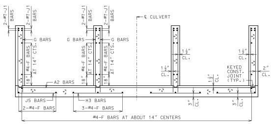
UPSTREAM AND DOWNSTREAM WINGS REINFORCEMENT
