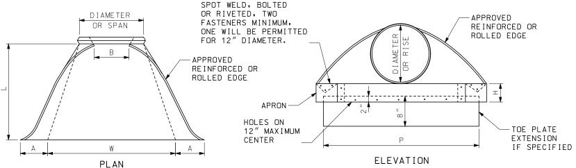
END SECTION FOR PIPE AND PIPE ARCH
