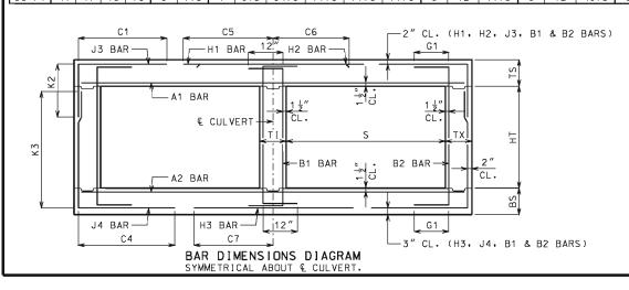
IF DESIGN FILL IS BETWEEN TABULATED DESIGN FILLS, USE THE NEXT GREATER TABULATED DESIGN FILL, EXCEPT FOR DESIGN FILLS BETWEEN 2 FEET AND 4 FEET. FOR DESIGN FILLS BETWEEN 2 FEET AND 4 FEET USE THE GREATER MEMBER THICKNESS, AREA OF REINFORCEMENT AND BAR DIMENSIONS FROM THE 2 FEET AND 4 FEET TABULATED DESIGN FILLS. AREA OF REINFORCEMENT EQUALS BAR AREA PER FOOT SPACING.
