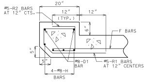
UPSTREAM HEADWALL REINFORCEMENT
