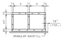
GRANULAR BACKFILL LIMITS AND MEMBER DIMENSIONS
