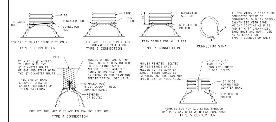
END SECTION FOR PIPE AND PIPE ARCH
