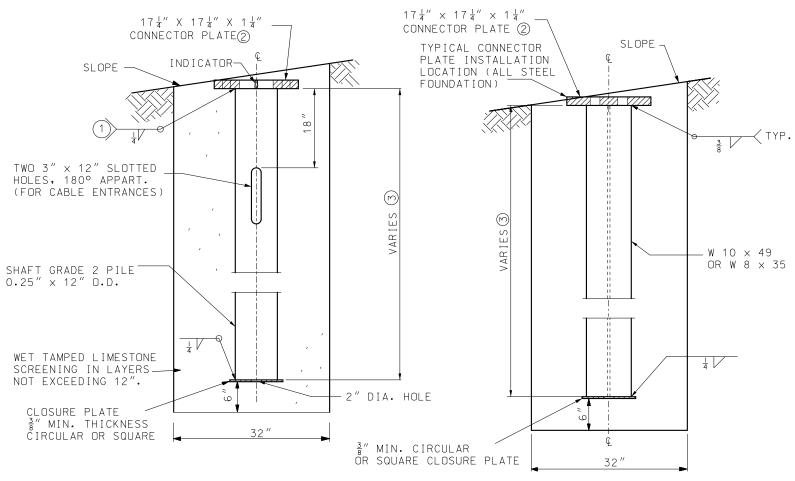
ELEVATION DETAILS OF CIRCULAR STEEL PILE FOUNDATION
