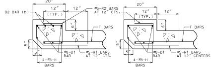
UPSTREAM HEADWALL REINFORCEMENT NEAR INTERIOR WALL
