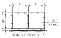
GRANULAR BACKFILL LIMITS AND MEMBER DIMENSIONS
