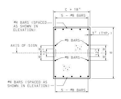
SECTION B-B TYPICAL SECTION SHOWING REINFORCING STEEL
