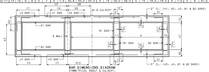
IF DESIGN FILL IS BETWEEN TABULATED DESIGN FILLS, USE THE NEXT GREATER TABULATED DESIGN FILL, EXCEPT FOR DESIGN FILLS BETWEEN 2 FEET AND 4 FEET. FOR DESIGN FILLS BETWEEN 2 FEET AND 4 FEET USE THE GREATER MEMBER THICKNESS, AREA OF REINFORCEMENT AND BAR DIMENSIONS FROM THE 2 FEET AND 4 FEET TABULATED DESIGN FILLS. AREA OF REINFORCEMENT EQUALS BAR AREA PER FOOT SPACING.
