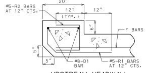
UPSTREAM HEADWALL REINFORCEMENT
