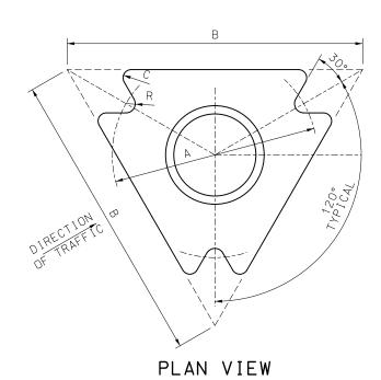
ROLLED CRIMP TO ENGAGE PIPE O.D.
