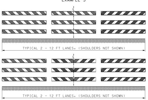
EXAMPLE 1 - ONE TYPE 3 MOVABLE BARRICADE WILL BE REQUIRED TO COMPLETELY CLOSE EACH 8' OF PAVEMENT. PAVED SHOULDERS SHALL BE INCLUDED IN THE AREA TO BE CLOSED.
