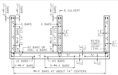
UPSTREAM AND DOWNSTREAM WINGS REINFORCEMENT
