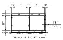
GRANULAR BACKFILL LIMITS AND MEMBER DIMENSIONS
