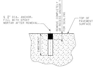
DETAIL SHOWING SEALING OF HOLES AFTER REMOVAL OF TIE-DOWN BOLTS
