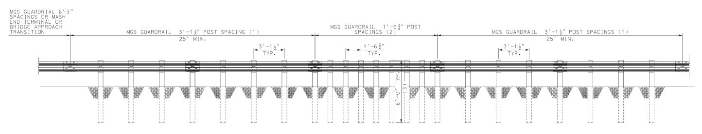
MGS GUARDRAIL WITH  $1'-6\frac{3}{4}"$ POST SPACING
