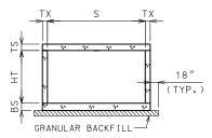
GRANULAR BACKFILL LIMITS AND MEMBER DIMENSIONS
