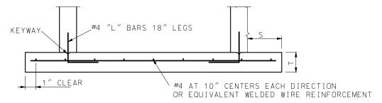
SECTION C-C S = 0 FOR DEPTHS LESS THAN OR EQUAL TO 6': S = 9" FOR DEPTHS GREATER THAN 6'.
