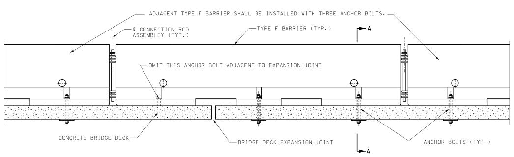
BOLT THROUGH DECK AT THERMAL EXPANSION JOINTS
