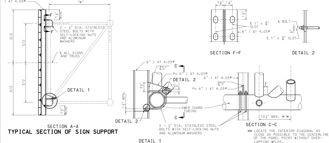
ALL SIGNS SHALL BE CENTERED VERTICALLY ABOUT THE HORIZONTAL  $\ensuremath{\mathbb{Q}}$  OF THE TRUSS.
