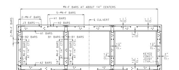
BARREL REINFORCEMENT FOR DESIGN FILLS OVER 2'-0"
