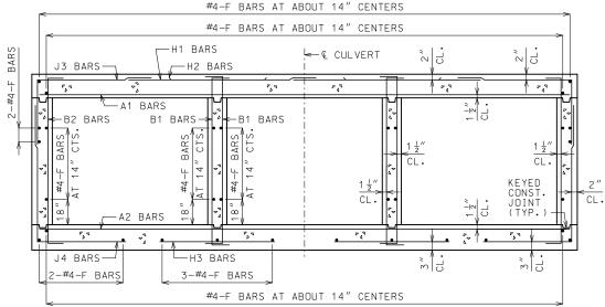
BARREL REINFORCEMENT FOR DESIGN FILLS 2'-0" OR LESS
