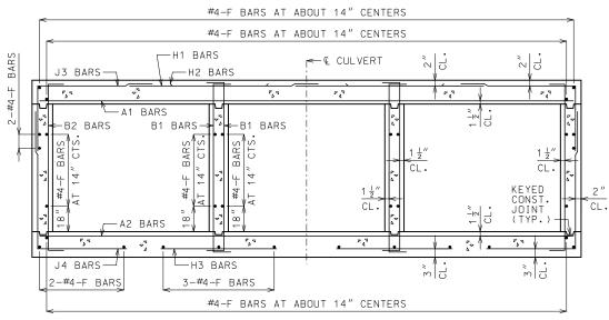
BARREL REINFORCEMENT FOR DESIGN FILLS 2'-0" OR LESS
