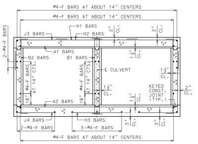
BARREL REINFORCEMENT FOR DESIGN FILLS 2'-0" OR LESS
