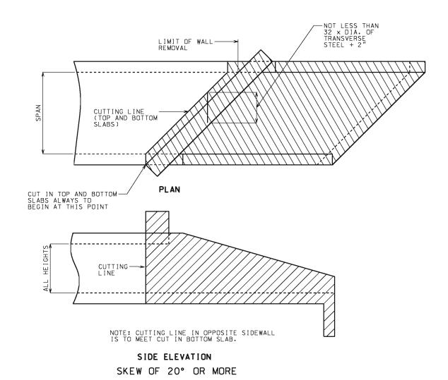
THE HATCHED PARTS OF THESE DRAWINGS INDICATE THOSE PORTIONS OF THE EXISTING CULVERT WHICH ARE TO BE REMOVED.
