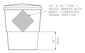
TYPE I OBJECT MARKER PLACEMENT FOR TEMPORARY INSTALLATIONS
