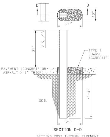
SETTING POST THROUGH PAVEMENT (CONCRETE OR ASPHALT > 2" THICK)
