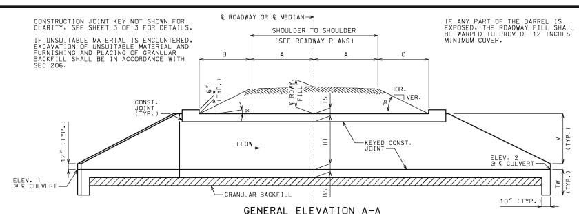
CHANNEL BOTTOM SHALL BE GRADED WITHIN RIGHT OF WAY FOR TRANSITION OF CHANNEL BED TO CULVERT OPENINGS. CHANNEL BANKS SHALL BE TAPÉRED TO MATCH CULVERT OPENINGS.
