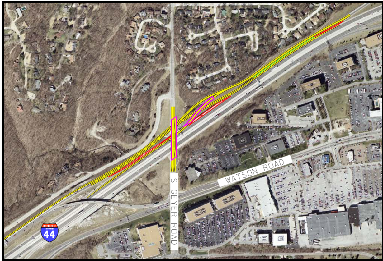
Figure 44: Westbound I-44 Braided Ramps between Lindbergh Boulevard and C-D Road
