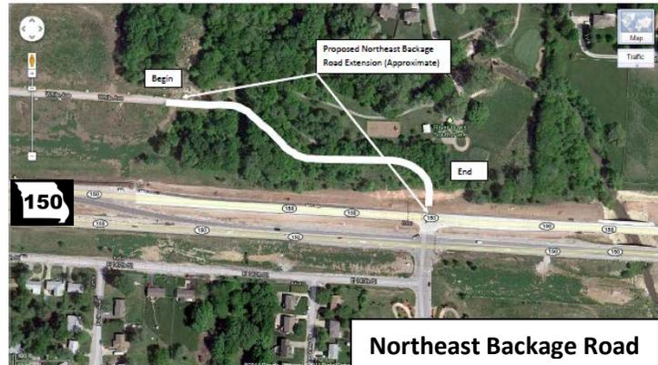
The Northeast Backage Road will be located in the northeast quadrant of the interchange. It will extend east from an existing unnamed dead end east/west road that intersects White Avenue on its west end, cross over Oil Creek, and turn south to intersect the north side of Mo 150 at the same location as Grand Summit Boulevard to the south.
