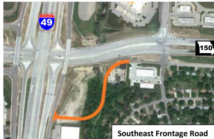
The Southeast Frontage Road Connector will be in the southeast quadrant of the interchange and will start at the East Route 71 Frontage Road and will extend east to connect to cross over the Little Blue River and connect to the west end of E. 147th Street.
