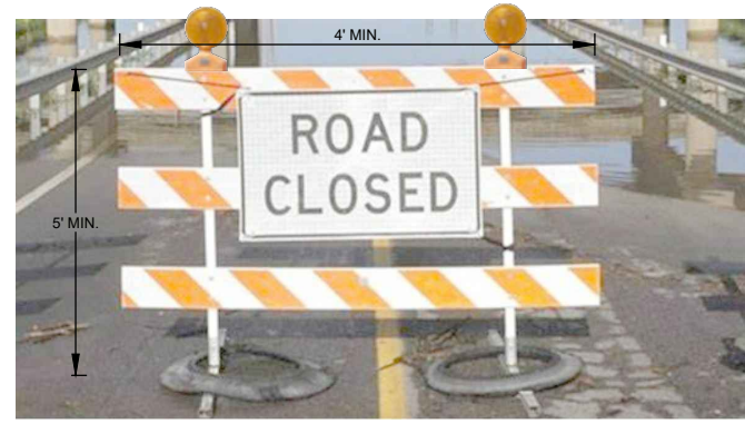
1 TYPE 3 MUTCD MOVEABLE BARRICADE W/ WARNING LIGHTS & ROAD CLOSED SIGN NOT TO SCALE
