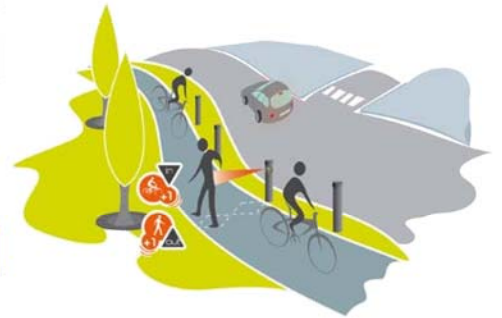
Example of an Eco-MULTI differentiating between cyclists and pedestrians on a shared area
