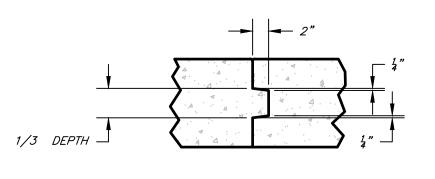
CONCRETE CONSTRUCTION JOINT DETAIL (IF REQUIRED)
