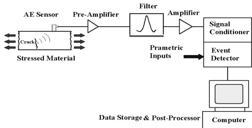
**Figure E-1. Schematic representation of Acoustic Emission testing setup**
