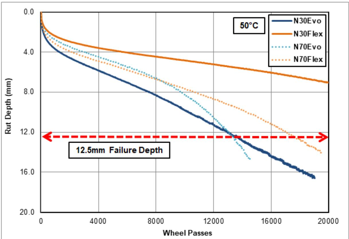
Figure D-42. Hamburg test results
