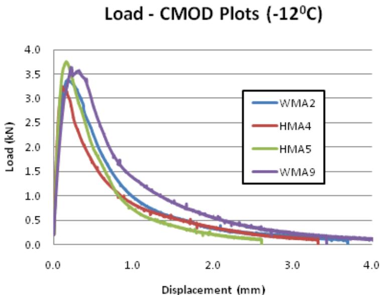
**Figure D-15. Typical DC(T) load-CMOD plots**
