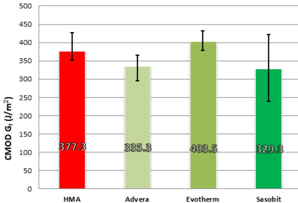
**Figure D-30. DC(T) results for virgin HMA and WMA mixtures**
