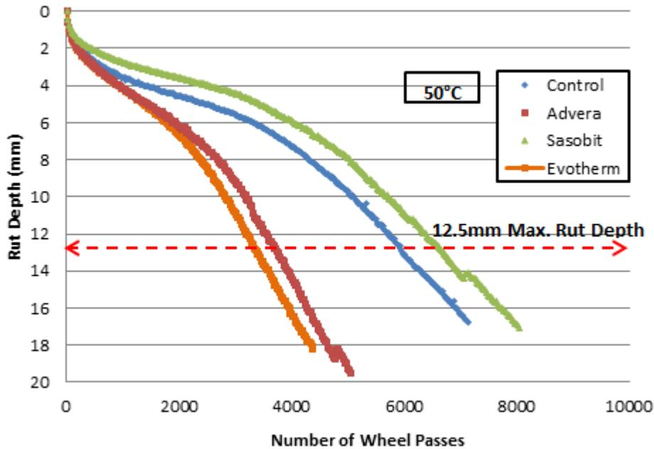
**Figure D-21. Virgin Mixture rut depth profiles**
