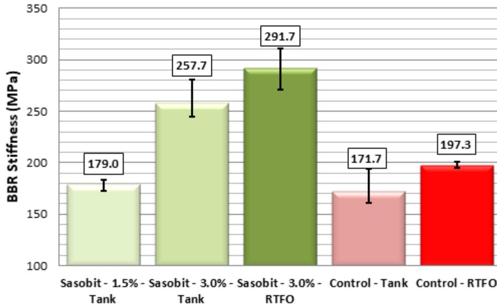
**Figure D-20. Sasobit tank and RTFO binder stiffness**
