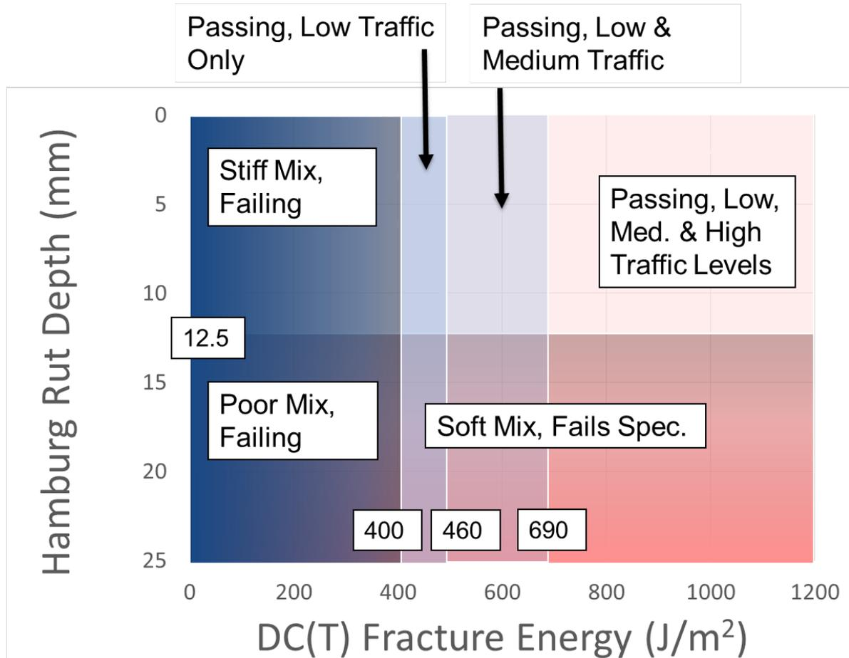
Figure D-45. Hamburg-DC(T) plot with typical specification limits superimposed
