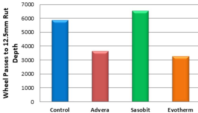
**Figure D-22. Virgin mixture wheel passes to maximum rut depth**
