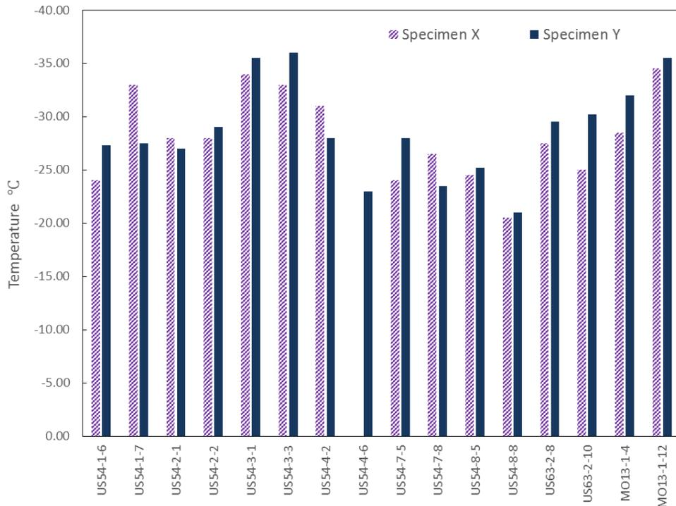
**Figure E-4. Embrittlement Temperatures of X and Y Specimens for all mixture samples**
