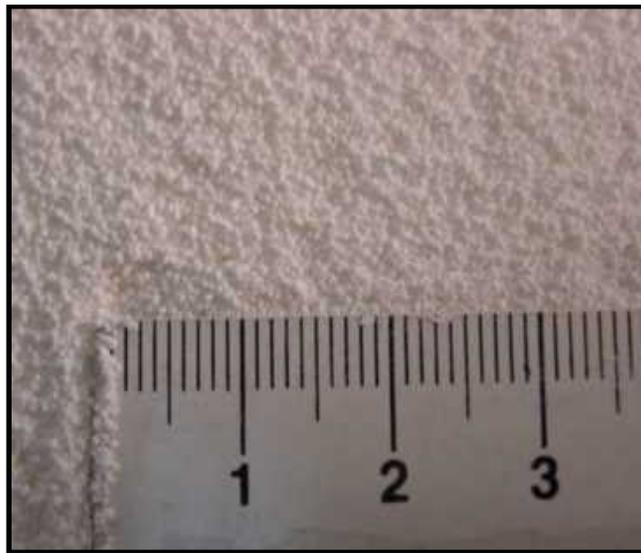
**Figure D-8. Aspha-min Zeolite**
