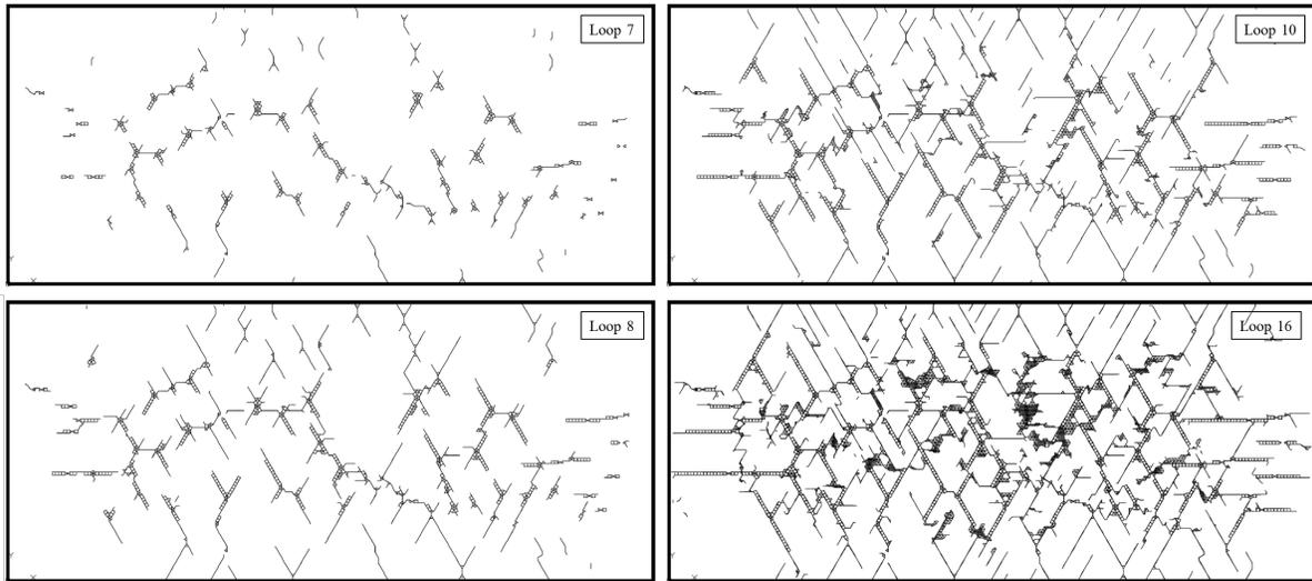
**Figure C-5. Crack propagation patterns at various stages in the DEM simulation**
