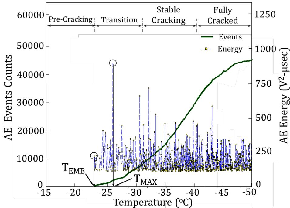
**Figure E-3. Typical AE test result for asphalt materials**
