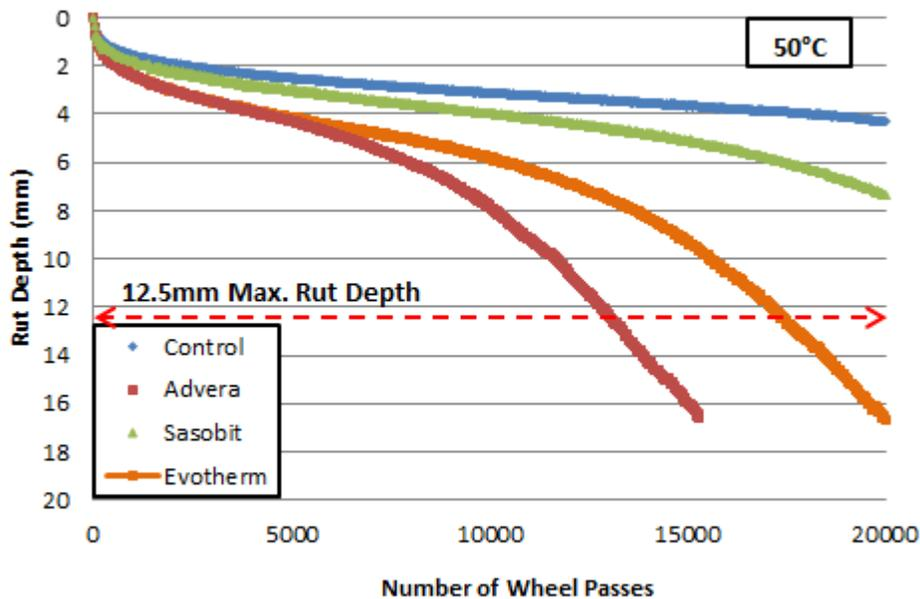
Figure D-24. 45% RAP mixture rut depth profiles
