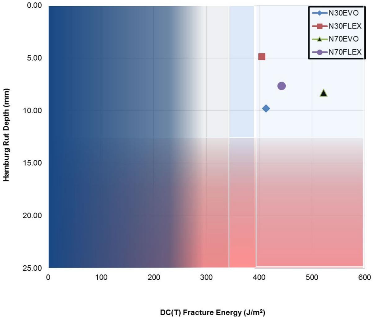
**Figure D-46. Hamburg-DC(T) plot for N70 CHI mixes and N30 reference mixes**
