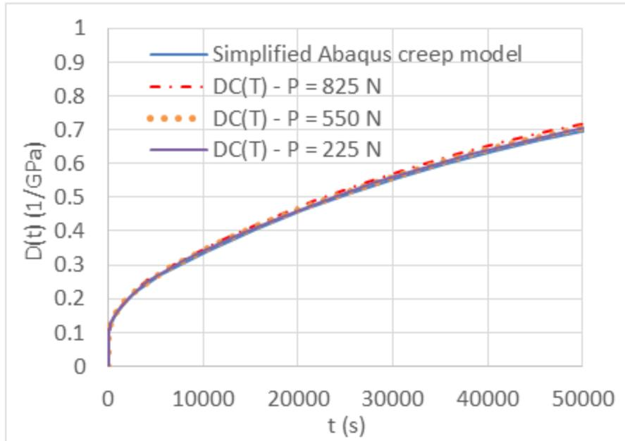
**Figure B-5. Creep compliance values obtained using Eq. (3) and based on simulation results obtained from 3D DC(T) models**
