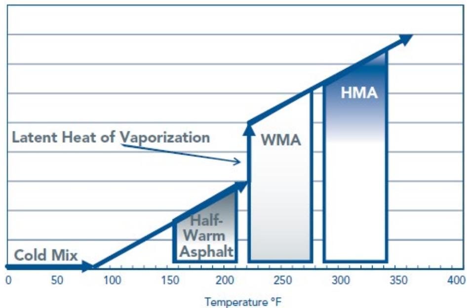
**Figure D-2. Production temperatures of asphalt concrete**
