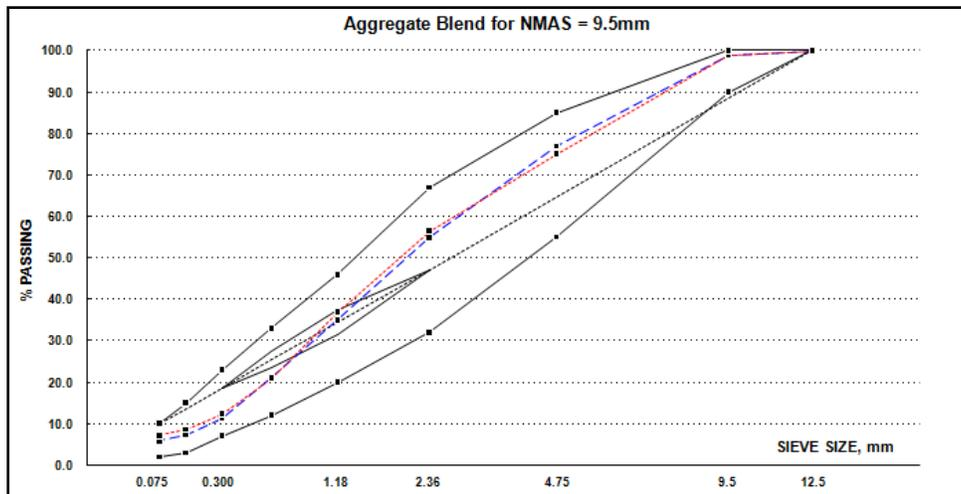
**Figure D-12. Virgin and 45% RAP mixture design gradations**
