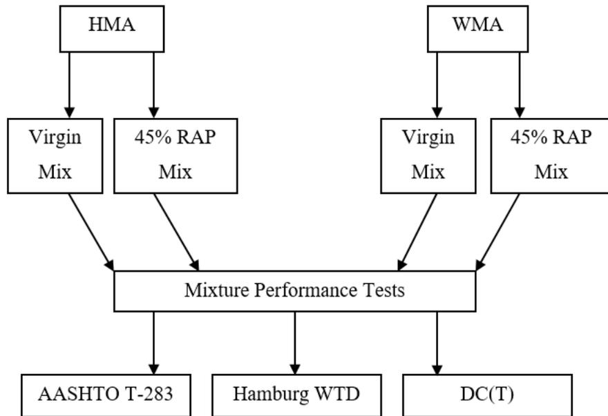
**Figure D-11. Mixture testing suite**
