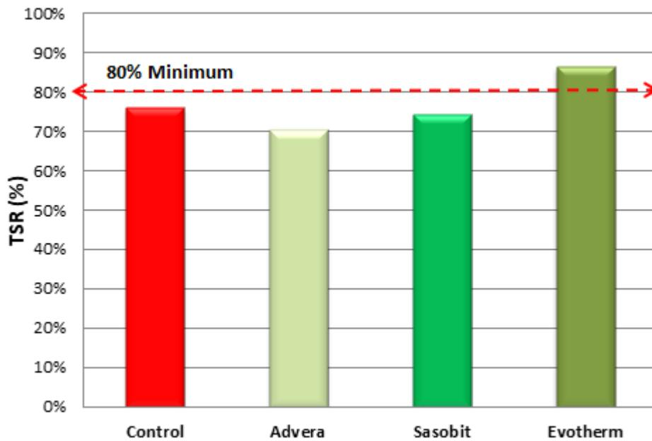
**Figure D-29. 45% RAP HMA and WMA mixture TSR results**
