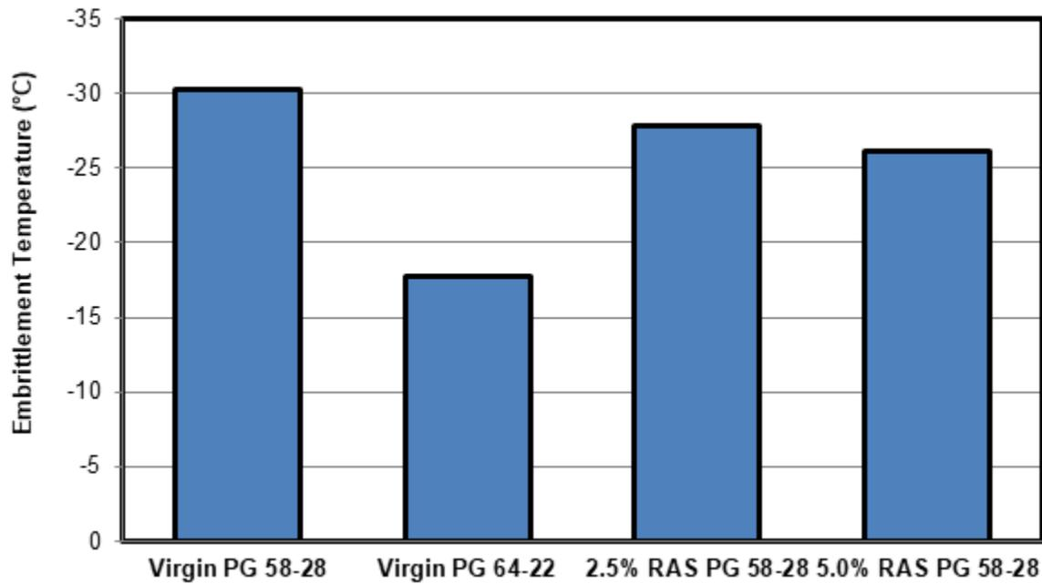
Figure D-37. Acoustic emission embrittlement temperature test results
