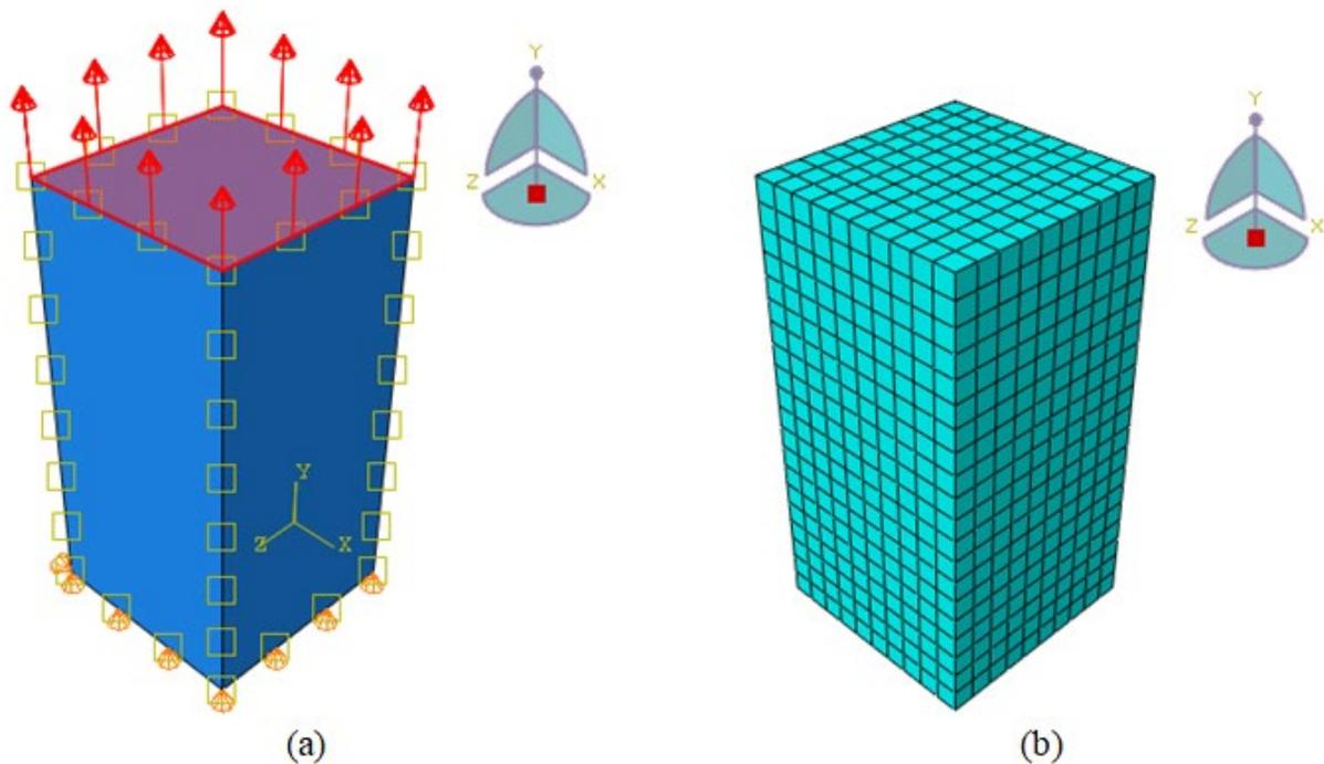
**Figure B-1. Simplified model used to verify creep and relaxation tests: (a) loading and boundary conditions and (b) finite element mesh**
