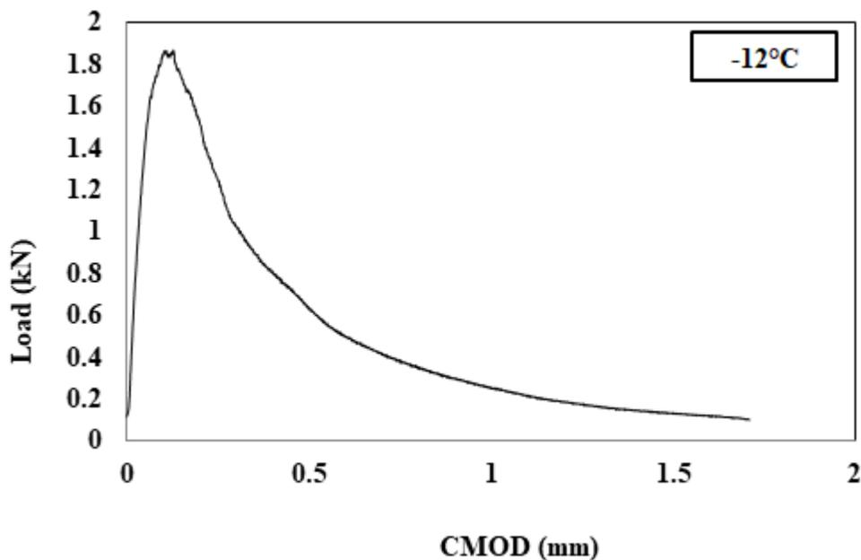
**Figure C-2. Load-CMOD curve of the surface mix**
