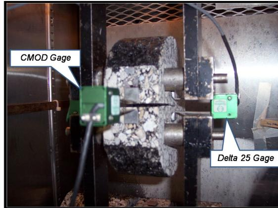
**Figure D-16. DC(T) testing arrangement**
