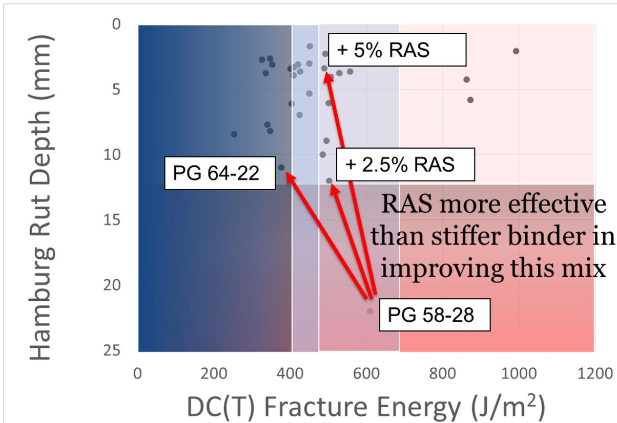
**Figure D-40. Hamburg DC(T) Plot showing typically Illinois’ mixture data, along with 4 data points collected in this study (located at the beginning and ends of red arrows)**
