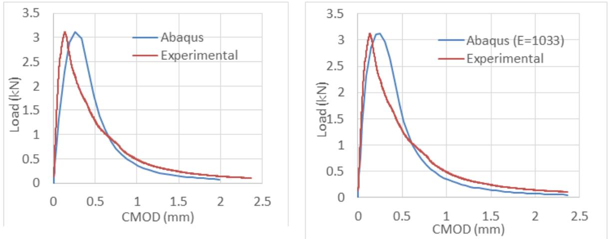
**Figure B-6. Numerical vs. Experimental fracture test results obtained using (a)  $E_{\infty}=0.741$  GPa (Table B-2) and (b)  $E_{\infty}=1.033$  GPa**
