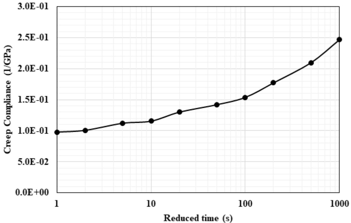
**Figure C-3. Creep compliance results from US63 La Plata field cores, at a reference temperature of -24°C**
