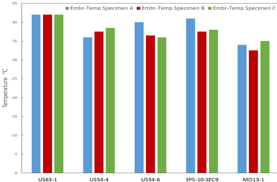
**Figure E-6. Embrittlement Temperatures in °C of A, B, C specimens for all binder samples. See Table 3.**
