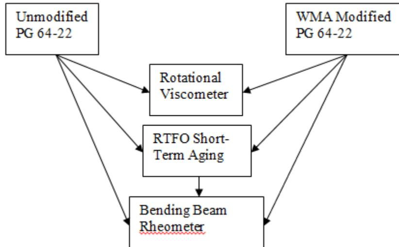
**Figure D-10. Asphalt binder testing plan**
