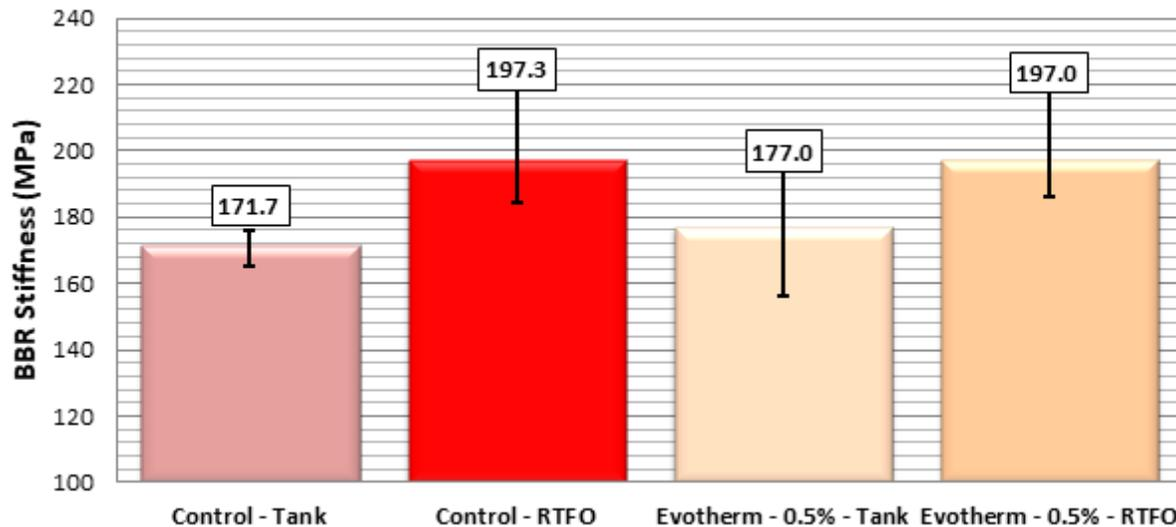
**Figure D-19. Evotherm tank and RTFO binder stiffness**
