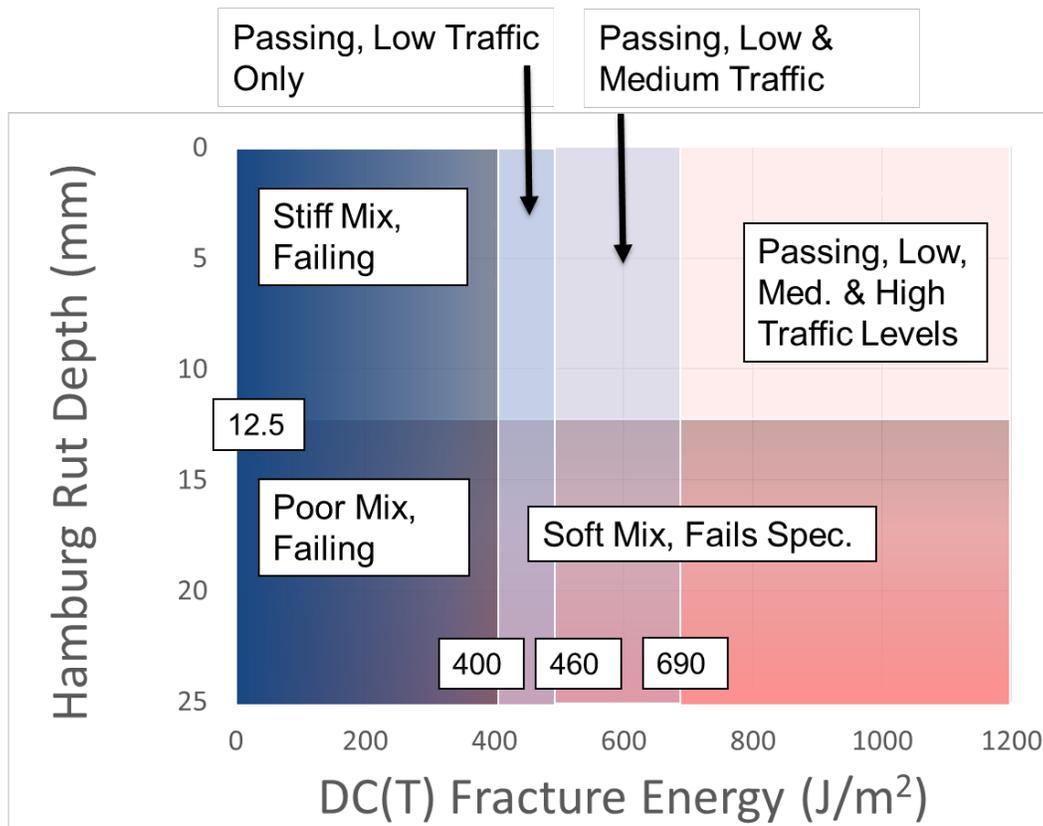
Figure D-39. Hamburg-DC(T) plot with typical specification limits superimposed
