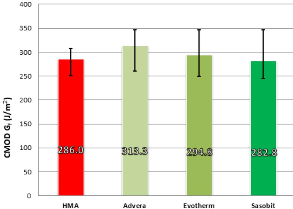
**Figure D-31. DC(T) results for 45% RAP HMA and WMA mixtures**
