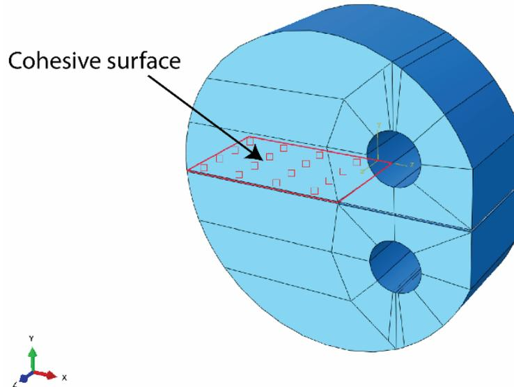
**Figure B-4. Cohesive fracture surface used to simulate fracture in the DC(T)**
