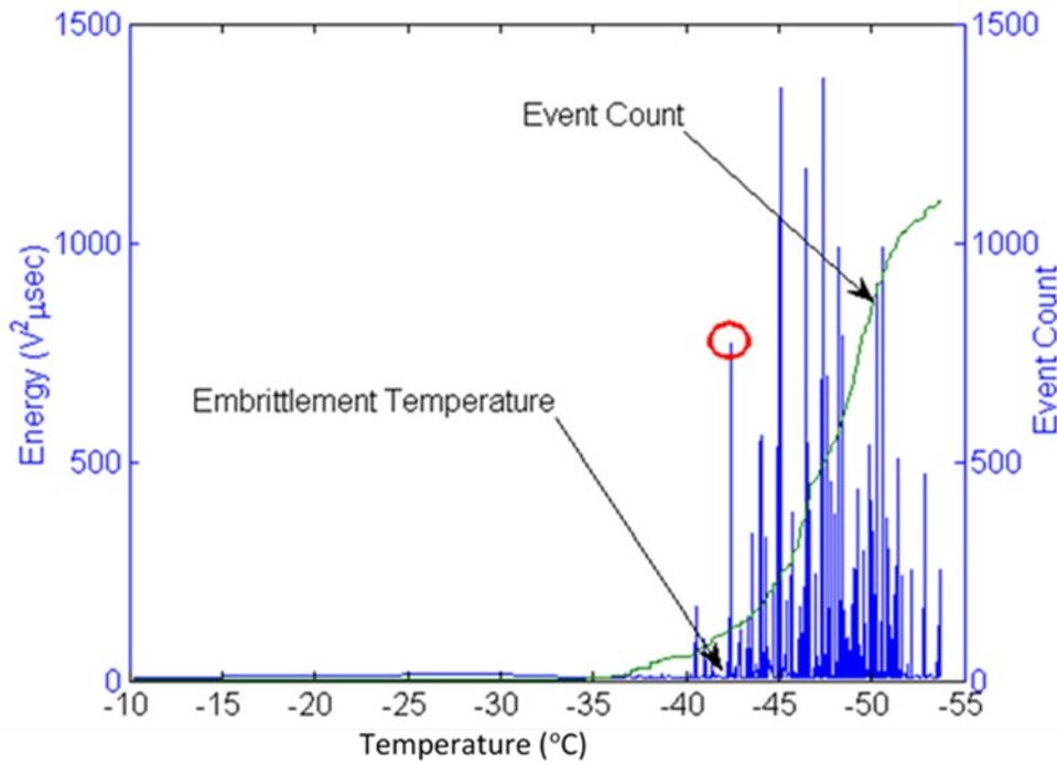
Figure E-7. Acoustic Emission Energy and Event Count versus Temperature for specimen B of US63-1 Binder Sample. Horizontal axis denotes temperature in °C.
