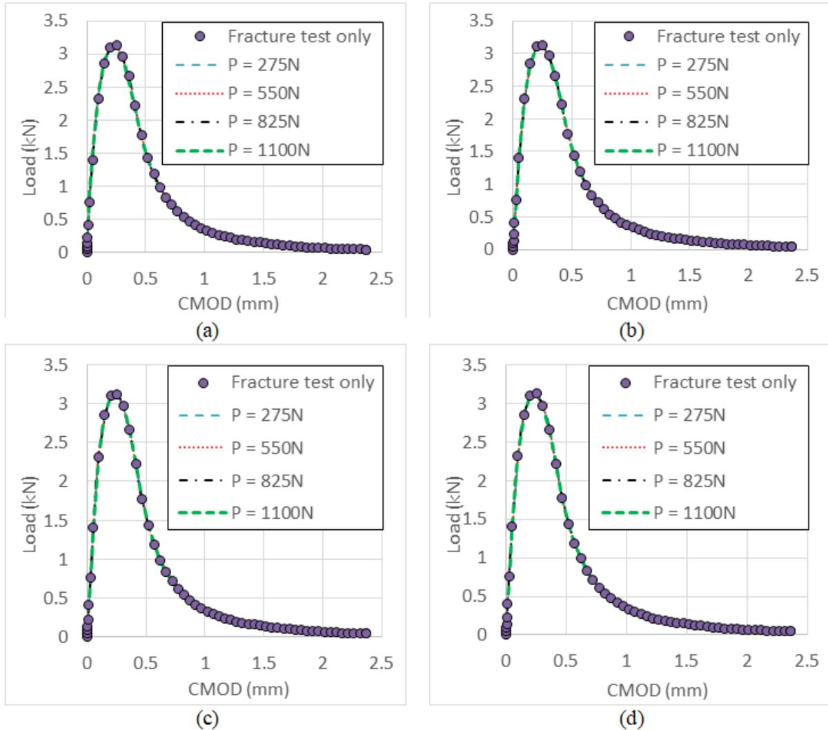
**Figure B-8. Results of simulated fracture tests obtained after conducting a creep/recovery test for rest times of (a) 0 hours, (b) 1 hour, (c) 12 hours, and (d) 24 hours**
