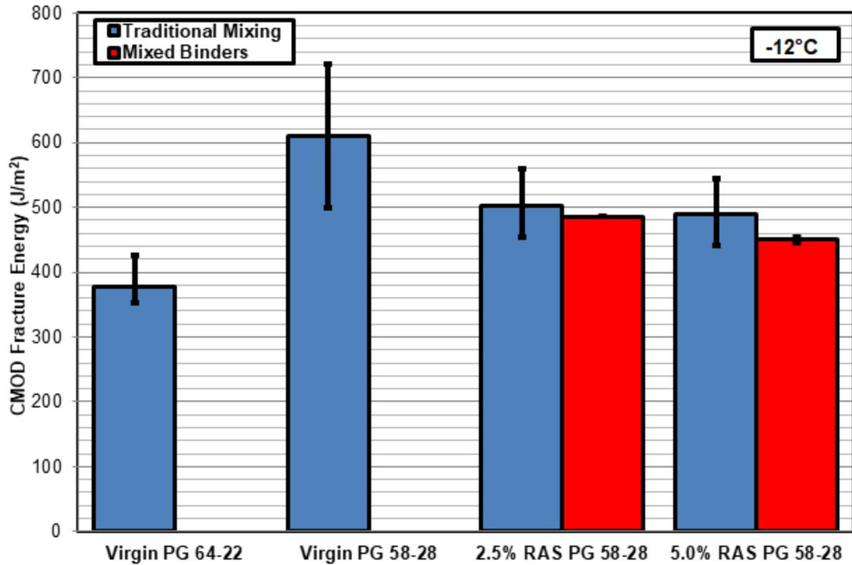
Figure D-36. DC(T) test results at -12°C
