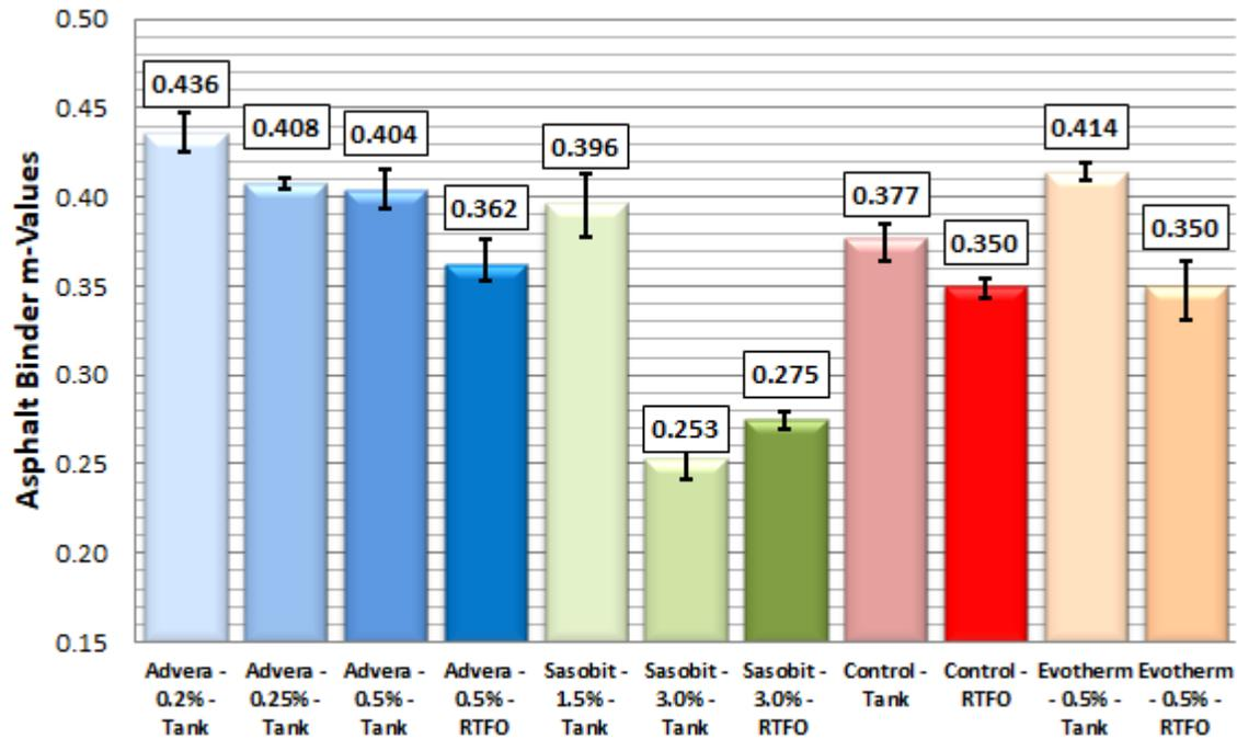
Figure D-17. Tank and RTFO binder M-Values
