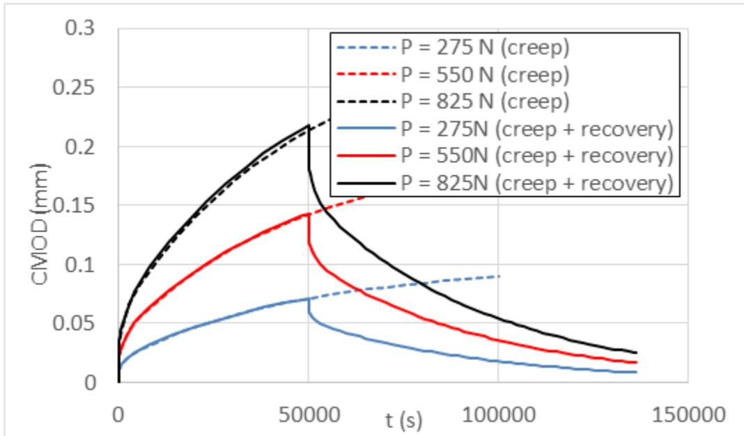
**Figure B-7. Simulated creep/recovery tests obtained from DC(T) models**
