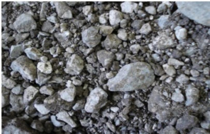
**Figure D-1. Reclaimed asphalt pavement (RAP)**
