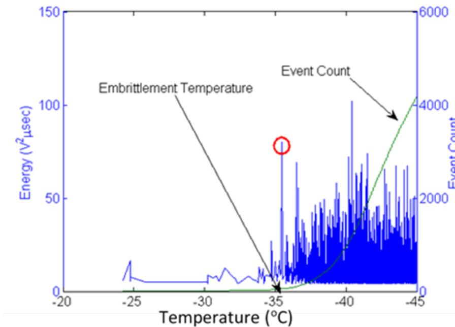
**Figure E-5. Acoustic Emission Energy and Event Count versus Temperature for specimen Y of US54-3-1 Sample. Horizontal axis denotes temperature in °C.**
