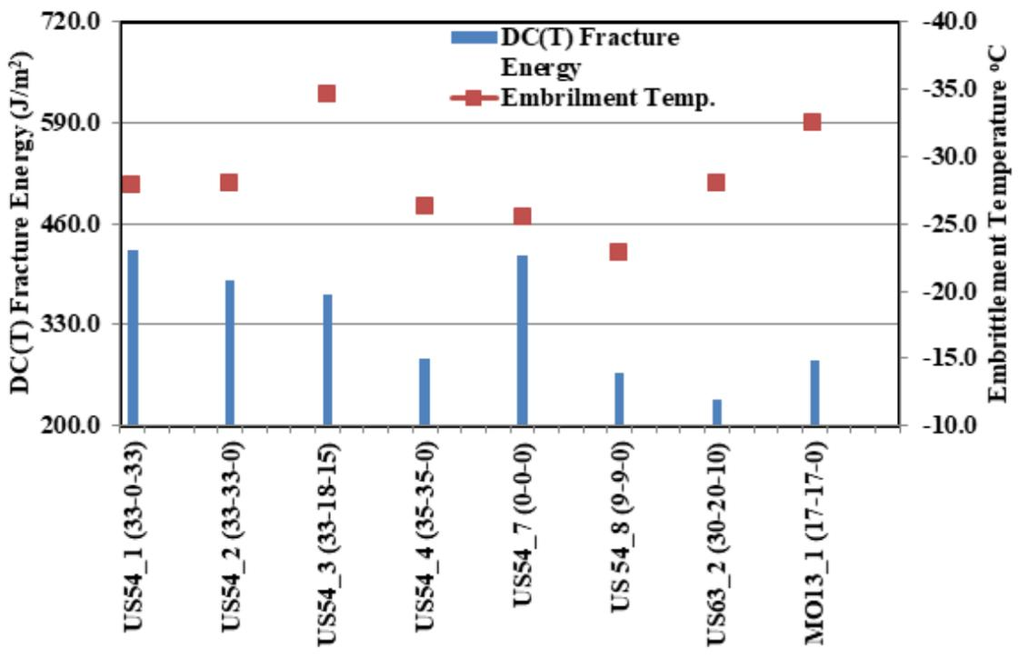
Figure E-8. Embrittlement temperature from Acoustic Emission test compared to the DC(T) fracture energy
