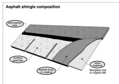
**Figure D-32. Asphalt shingle composition**
