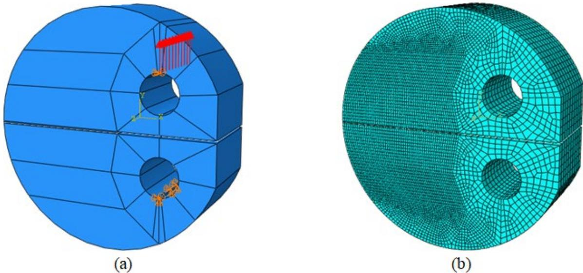
**Figure B-3. Three-dimensional DC(T) model used for simulation of creep compliance test:
