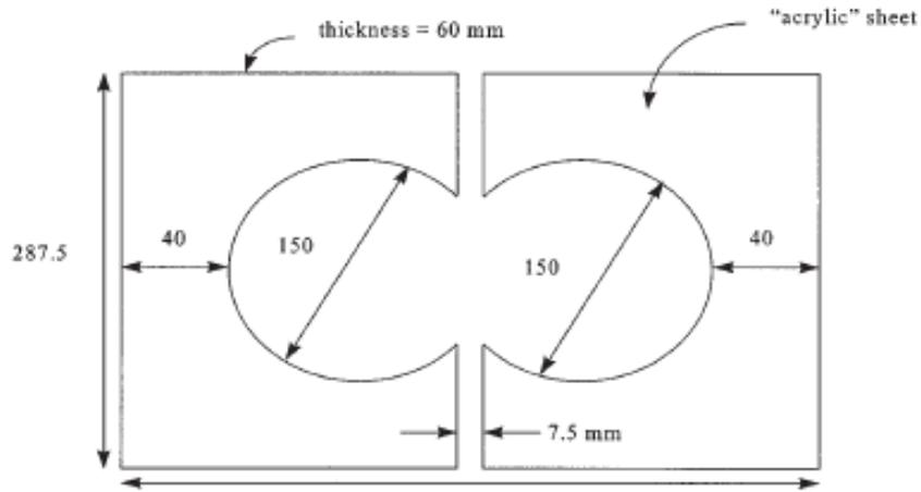
**Figure D-14. Hamburg gyratory specimen molds**
