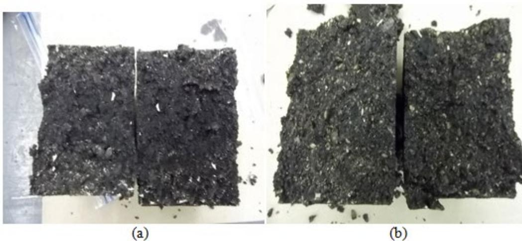
**Figure D-28. (a) Unconditioned Evotherm TSR sample and (b) Conditioned Evotherm TSR sample**
