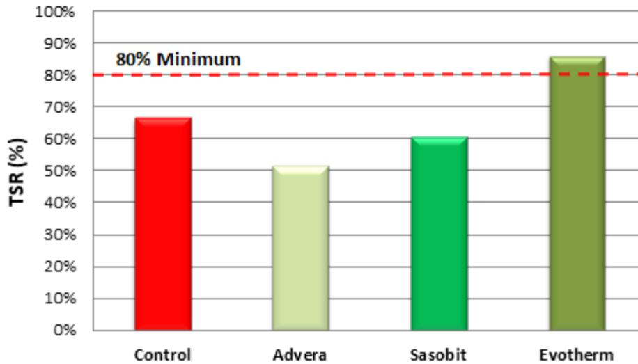
**Figure D-27. TSR results for virgin HMA and WMA mixtures**
