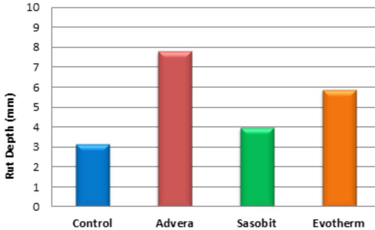
Figure D-25. 45% RAP mixture rut Depths at 10,000 wheel passes
