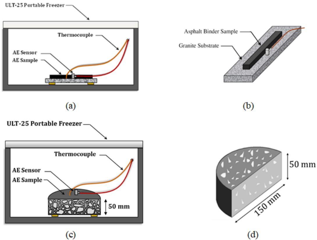
**Figure E-2. (a) AE testing setup for asphalt binders (b) AE asphalt binder sample (thin film of asphalt binder bonded to granite substrate) (c) AE testing setup for asphalt mixtures (d) AE asphalt mixture sample**
