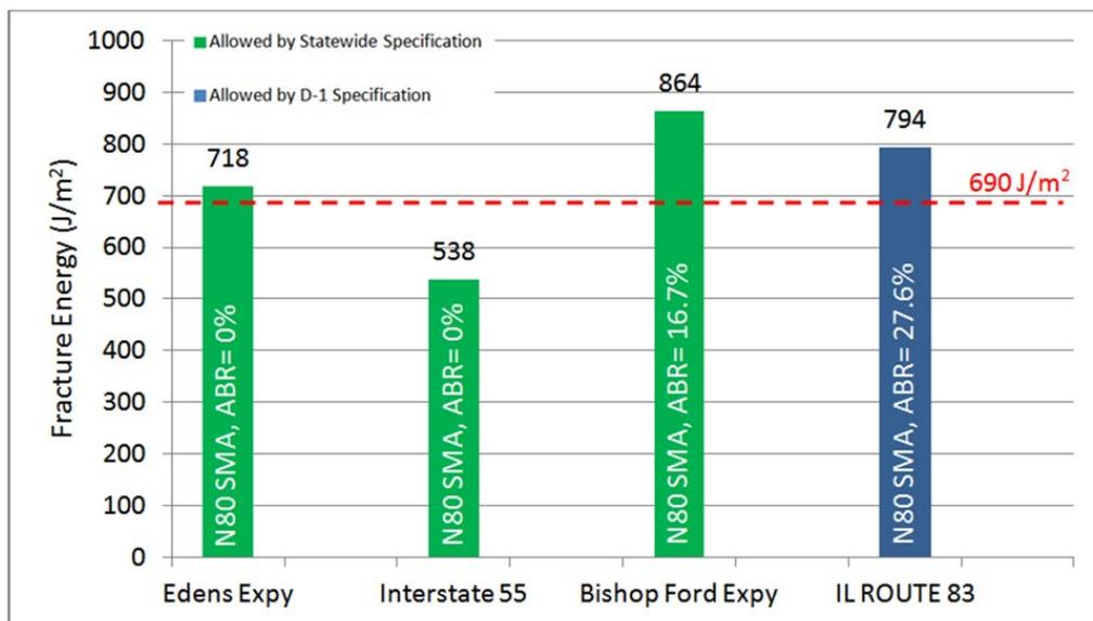
**Figure D-35. Sample fracture energy results from cores tested in DC(T): High traffic SMA mixes**
