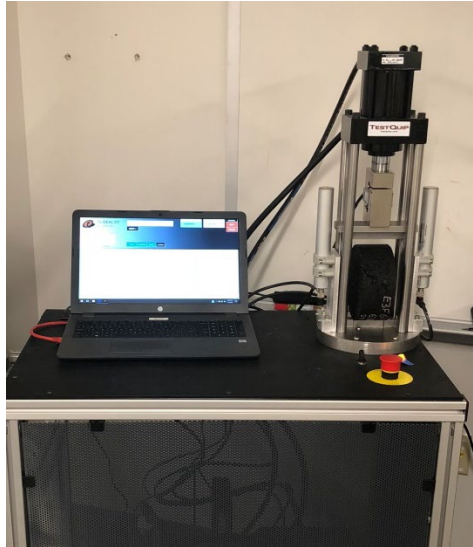
Figure 3-7. The Test Quip IDEAL-CT apparatus at MAPIL
