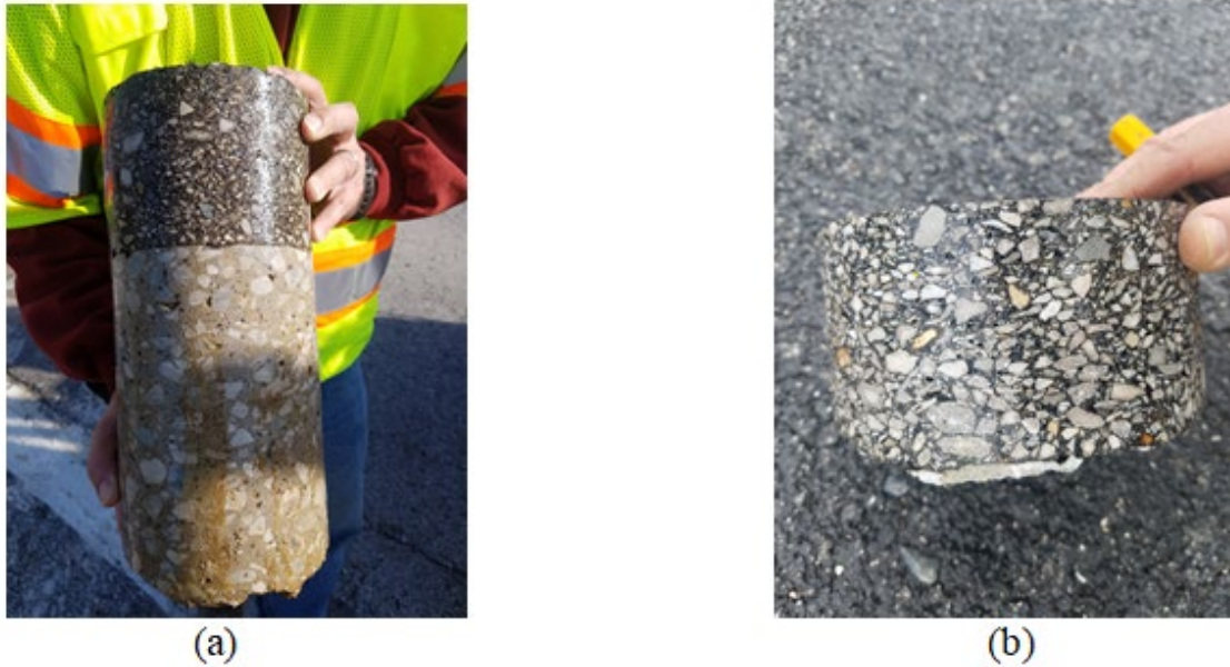
Figure 2-3. Example of project coring: (a) Full-depth core; (b) Asphalt layers only
