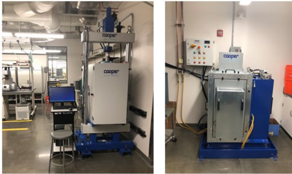
Figure 3-10. Cooper 100kN UTM machine at MAPIL
