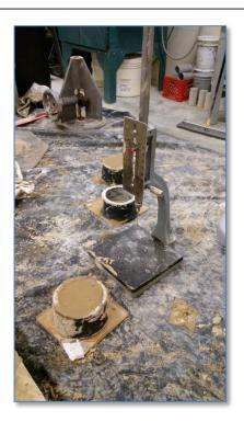
Setting time testing of zero-cement mortar
