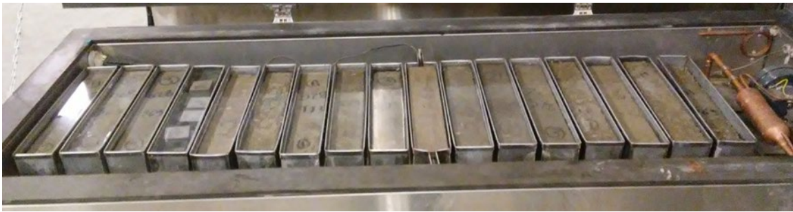
Figure 7.2: Freeze and thaw chamber for procedure A of ASTM C666-15 [74].
