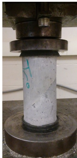
Figure 8.5: Slant shear test for the repaired cylinders.
