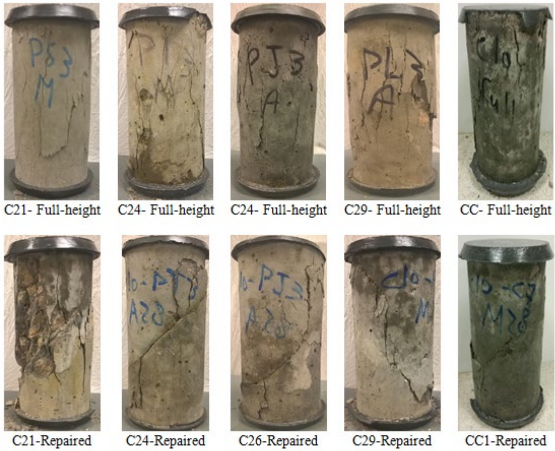
Figure 8.10: Failure modes of the full-height and repaired cylinders for the moist-cured specimens.
