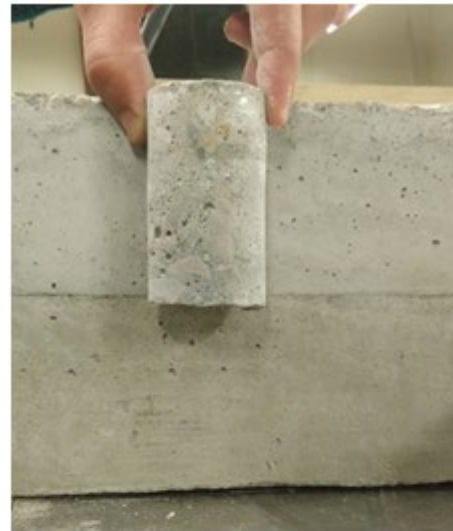
(b) Failure at the interface between the host and repair material
