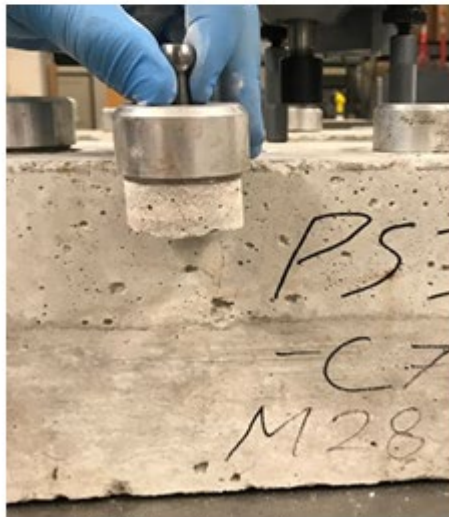
(c) Failure in repair material
