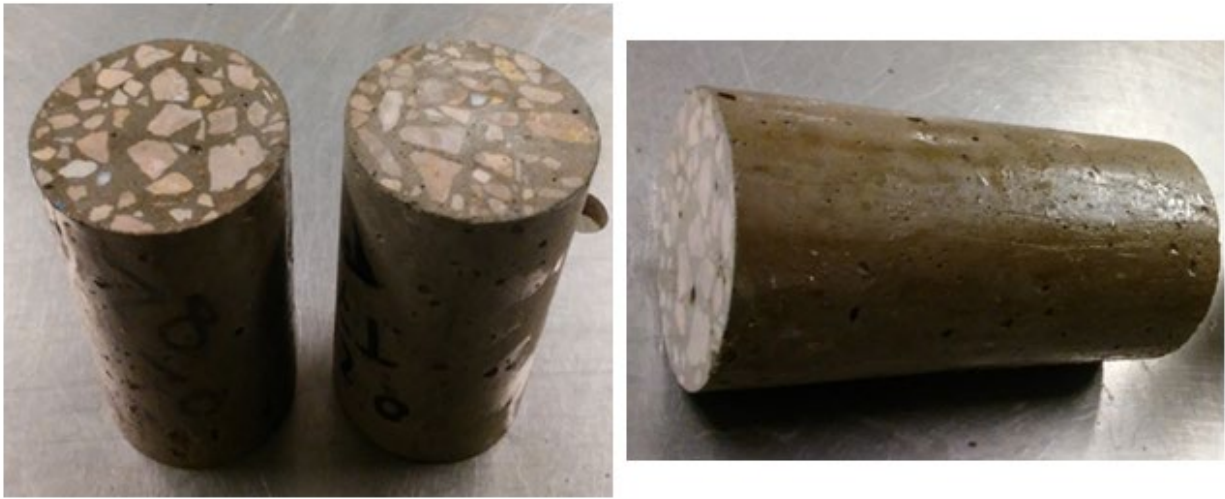
Figure 7.5: Grinded surfaces of the test specimens prior to the bulk electrical conductivity test.
