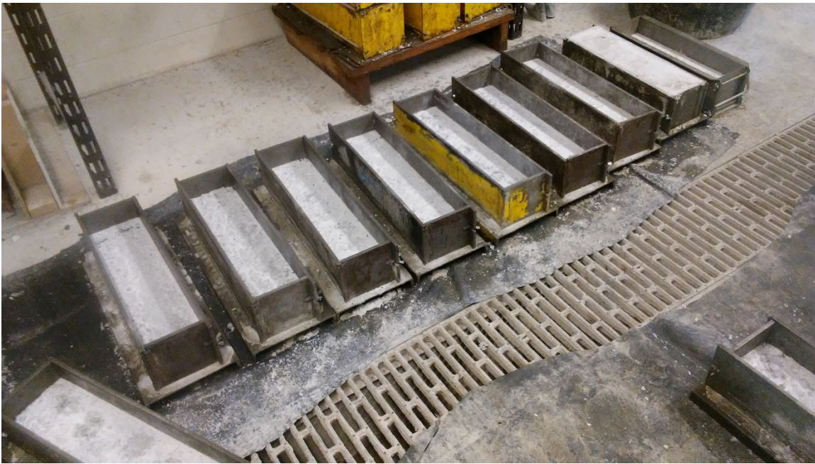
Figure 8.4: Half beams constructed out of the host material, i.e., CC after curing and before placing the ZCC repair.
