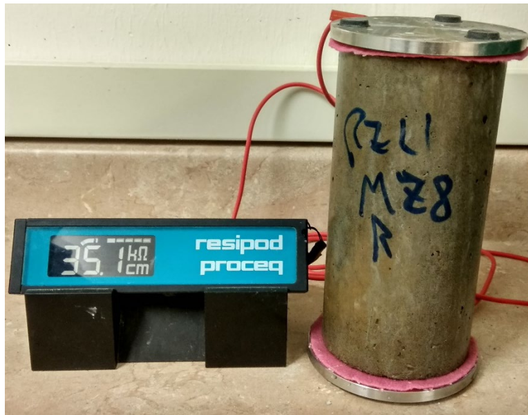
Figure 7.5: Grinded surfaces of the test specimens prior to the bulk electrical conductivity test.
