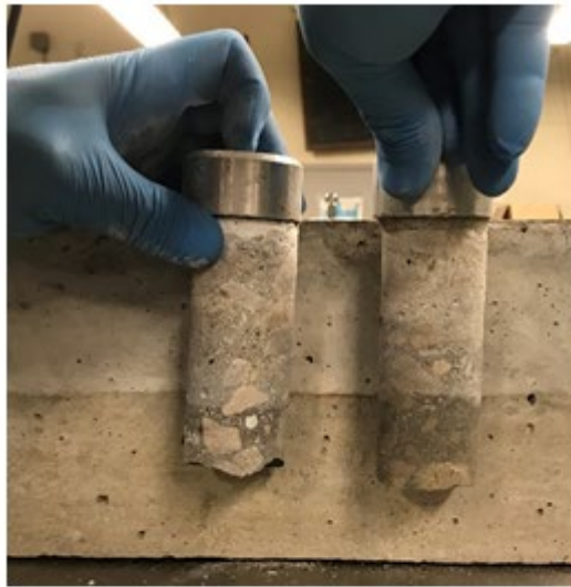
(a) Failure in the host CC material
