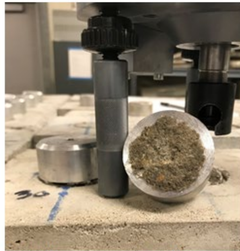
(d) Failure at top surface of the repair material
