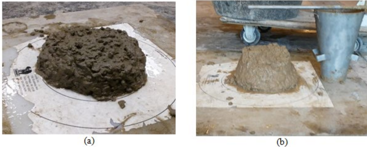
Figure 3.11: Examples of slump tests of ZCC (a) 8 in (mix 11 of FA27), and (b) 6.5 in (mix 7 of FA25).
