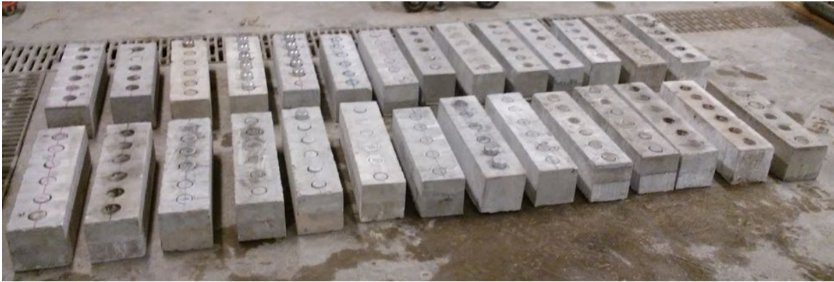
Figure 8.18: Beams tested for the pull-off test.
