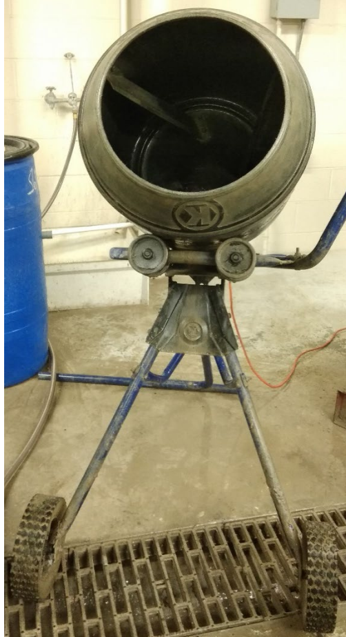
Figure 3.10: Gravity mixer with a maximum capacity of 1.5 ft 3 .
