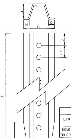
HOLE PUNCHING TO EQUAL 3" INCH DIAMETER HOLES, ONE INCH CENTER TO CENTER, BEGINNING ONE INCH FROM THE END AND CONTINUING THE ENTIRE LENGTH OF THE POST.
