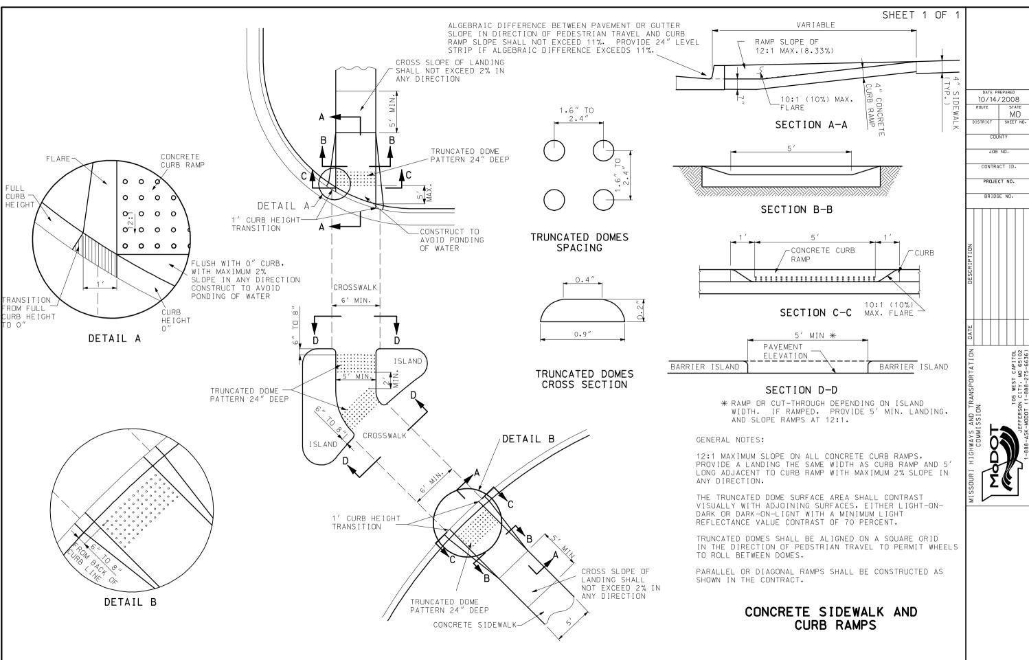
PERPENDICULAR CONCRETE CURB RAMP
