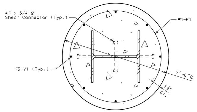
**SECTION SHOWING PILE ENCASEMENT WITH PARTIAL PILE REPLACEMENT**
