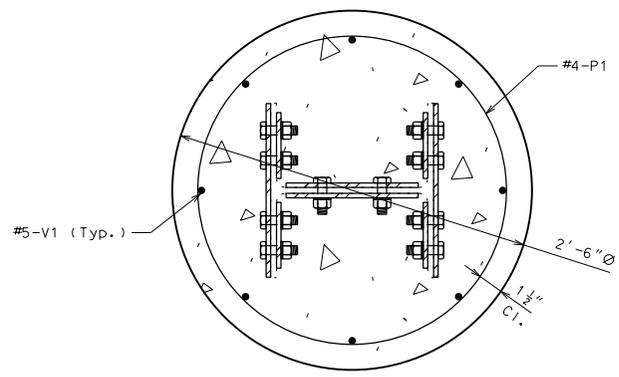
**SECTION SHOWING PILE ENCASEMENT WITH PILE PLATING**
