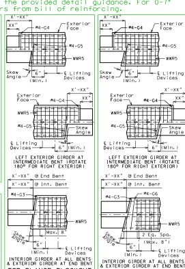
The left advanced details shown may be used for right advanced bridges. May remove mirror note if left advanced.
