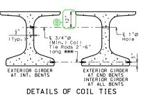
Cast 1"0 hole horizontally in girder for #6 bar 5'-6" long and clear reinforcing steel or strands by 1 1/2" minimum.
