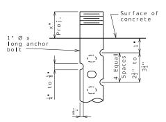
SWEDGE ANCHOR BOLT DETAIL
