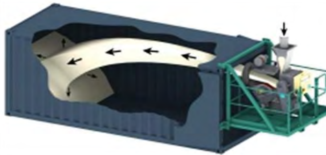
Figure J-10: Belt Thrower Loading Bulk Commodities
