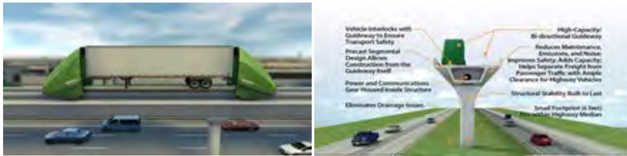
Figure 12: Freight Shuttle System Autonomous Transporter and Guideway
