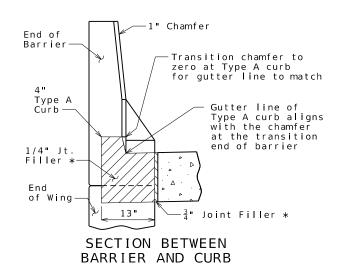
ALTERNATE DETAILS FOR TYPE B BARRIER (SBC)
