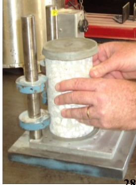
Capping with Sulfur Mortar
