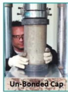
Un-Bonded Cap Unbonded caps ASTM C 1231
