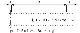
ELEVATION SHOWING SHEAR CONNECTOR SPACING FOR END BEAMS
