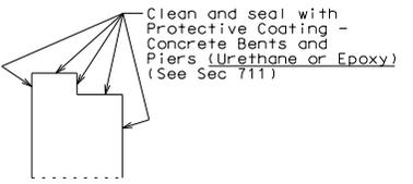
TYPICAL SECTION THRU INT. BENTS 2 & 3 SHOWING PROTECTIVE COATING
