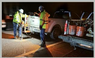
Pavement core samples of I-70 for design work.
