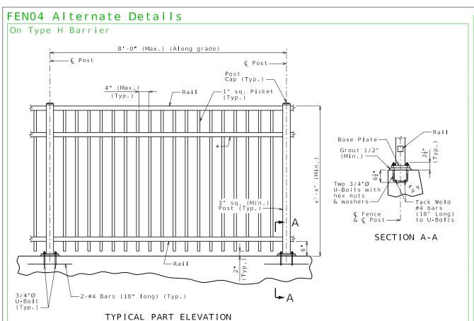
\* Optional rail. Need is based on design computations performed by the manufacturer and approved by MoDOT, or may be added for aesthetics.
